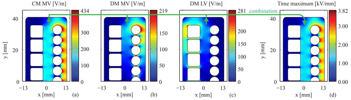
Fig. 6. Electric field for a CM excitation (1 V) of the MV winding (a), DM excitation ( $[-0.5 \text{ V}, 0.5 \text{ V}]$ ) of the MV (b), and LV (c) windings. The combination of (a-c) with the voltage excitations gives the maximal field in time domain (d). Since all fields are symmetrical, only half of the winding window is shown in each case.
