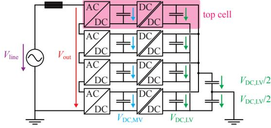
Fig. 1. One phase of the considered SST topology where each cell has an AC-DC and a DC-DC converter. The top cell is located at the MV end of the stack and is particularly important for insulation considerations.
