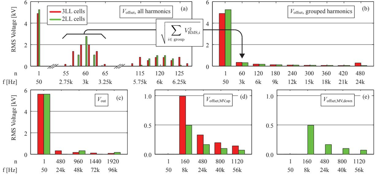
Fig. 5. RMS value of voltage harmonics for the cell placed at the top of the stack for all harmonics (a), and for grouped representation (b-e).
