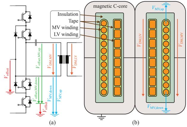
Fig. 3. Definition of the voltages within the MF transformer (top cell) (a), and cross-sectional view of the winding window of the transformer (11 : 8 ratio) with the corresponding insulation (b).
