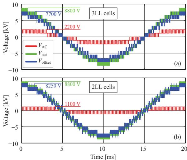
Fig. 4. Voltage waveforms in time domain for the top cell with 3LL (a) and 2LL (b) cells.
