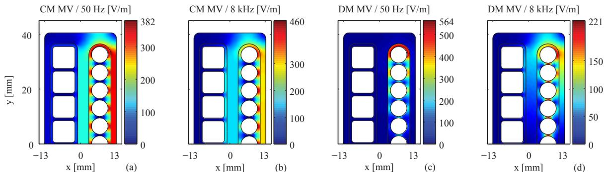
Fig. 13. Electric field for a CM excitation (1 V) of the MV winding (a-b) and DM excitation ( $[-0.5 \text{ V}, 0.5 \text{ V}]$ ) of the MV winding (c-d). The insulation system with semiconducting tapes is shown at 50 Hz and 8 kHz. Since the fields are symmetrical, only half of the winding window is shown.
