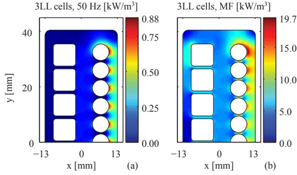
Fig. 9. Loss density for the grid frequency (a) and MF components (b) with 3LL cells. For saving space, only the upper part (where the losses are larger) of the winding window is shown even if the losses are not symmetrically distributed.
