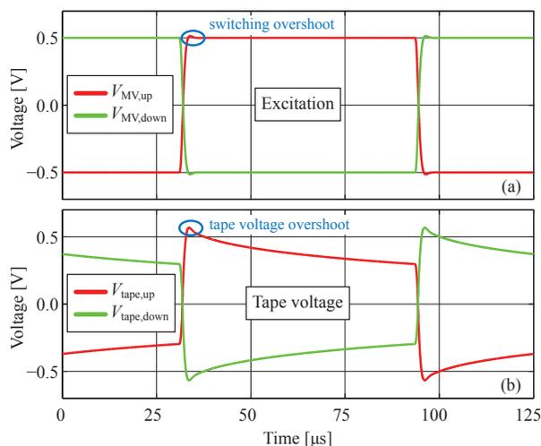
Fig. 14. DM excitation of the MV winding (a) and the corresponding voltage drop of the semiconducting tape (b). The voltages  $V_{MV,up}$  and  $V_{MV,down}$  are defined in Fig. 3, whereas  $V_{tape,up}$  and  $V_{tape,down}$  are the voltages extrema (maximum of the absolute value) along the tape near the upper and lower half of the winding window. The switching frequency is 8 kHz and the switching transitions are modeled with a small overshoot (1  $\mu\text{s}$  rise time).
