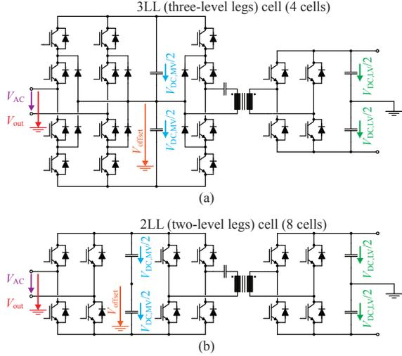
Fig. 2. Two possible realization options for the cascaded converter cells (top cell) based on three-level bridge legs (a) or two-level bridge legs (b).
