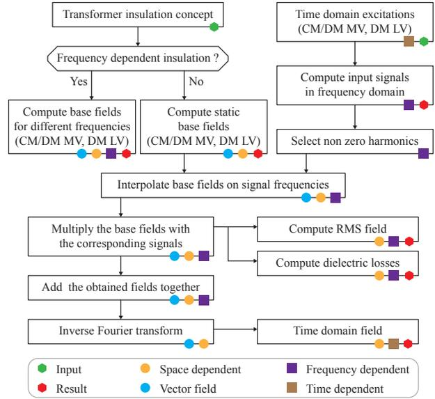
Fig. 11. Flow chart showing the computation method for analyzing a static or frequency-dependent insulation system in frequency and time domain.
