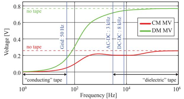
Fig. 12. Maximal voltage difference along the semiconducting tape (MV winding) for CM excitation (1 V) and a DM excitation ( $[-0.5 \text{ V}, 0.5 \text{ V}]$ ). The dashed curve represents the voltage drop along the tape when it has not been activated (tape with a zero conductivity).
