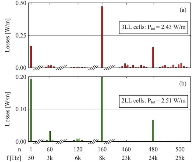
Fig. 10. Spectral distribution of the transformer dielectric losses for 3LL (a) and 2LL (b) cells.
