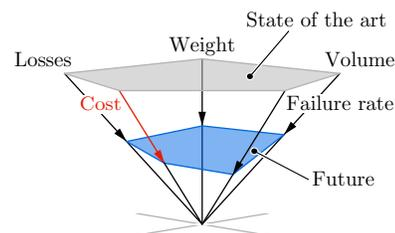
Fig. 1: Trends for performance improvements in the field of power electronics. Whereas the optimization of converter losses, weight and volume has been a major topic in research publications, cost and reliability issues have generally not yet been widely discussed. Considering this a motivation, this paper focuses on the analysis and modeling of the component costs of switched-mode power electronics converter systems.
