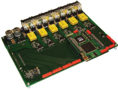
**Fig. 8:** Implemented bearing inverter system prototype.
