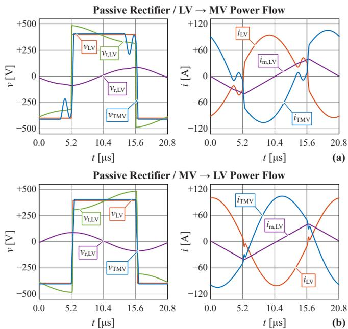
Fig. 5. Simulated voltages and currents with a passive rectifier bridge ( $f_s = 48\text{kHz}$  and  $P = 25\text{kW}$ ). (a) The power flow is directed from the LV bridge (active) to the MV bridge (passive). (b) The power flow is directed from the MV bridge (active) to the LV bridge (passive).
