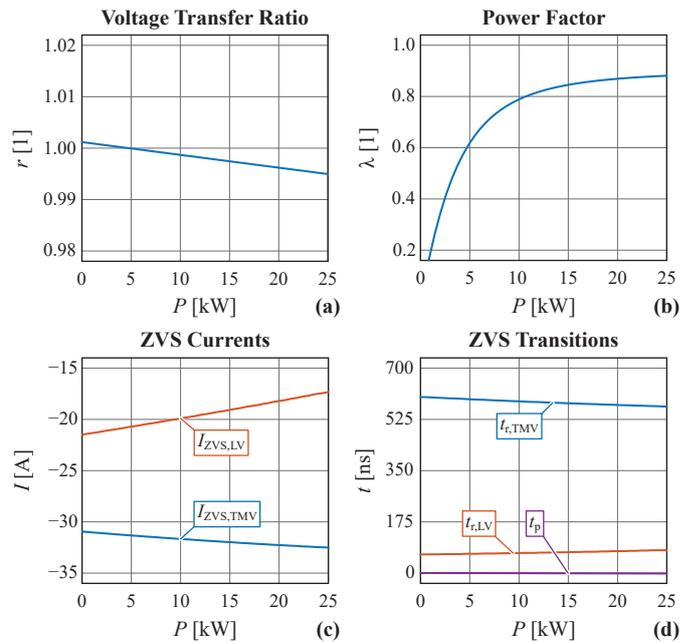
Fig. 14. Simulated (a) voltage transfer ratio (cf. (5)), (b) power factor (cf. (6)), (c) ZVS currents (average over the switching durations), and (d) ZVS transition durations. The phase shift between the bridge voltages is also shown (computed between the first Fourier harmonics). The SRC-DCX is operated with MCS-ZVS modulation ( $f_s = 48$  kHz,  $t_d = 270$  ns,  $P = 25$  kW, and power flow from the LV to the MV-side) at different load conditions.
