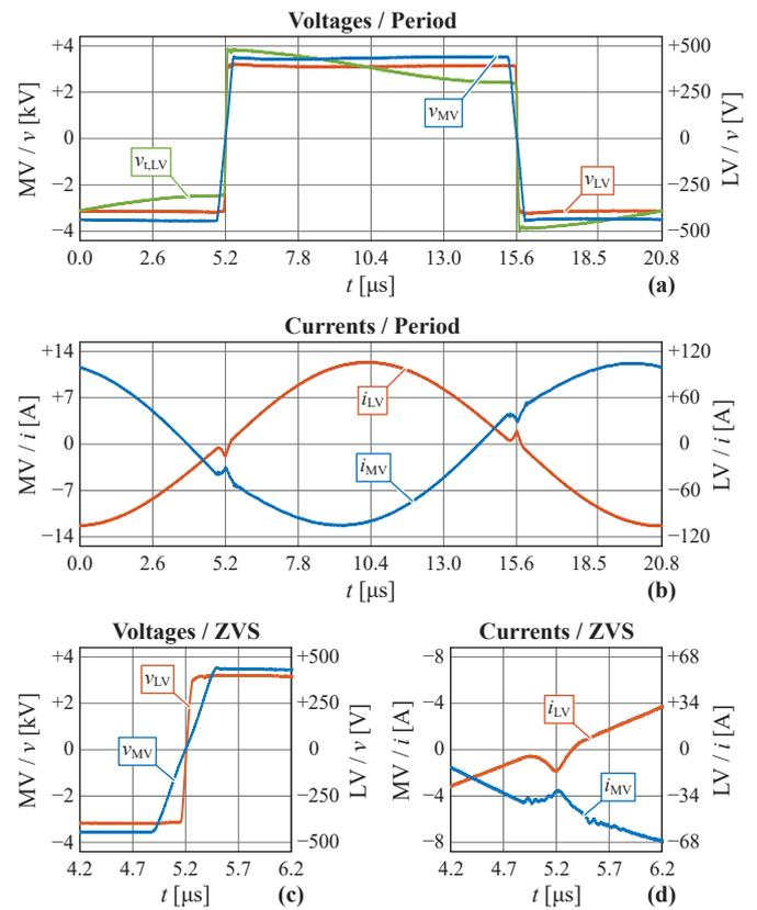
Fig. 16. Measured (a) voltages and (b) currents for a complete switching period. Measured (c) voltages and (d) currents during the ZVS transitions. The MCS-ZVS modulation ( $f_s = 48$  kHz,  $t_p = 270$  ns,  $P = 25.3$  kW, and power flow from the LV to the MV-side) is used.
