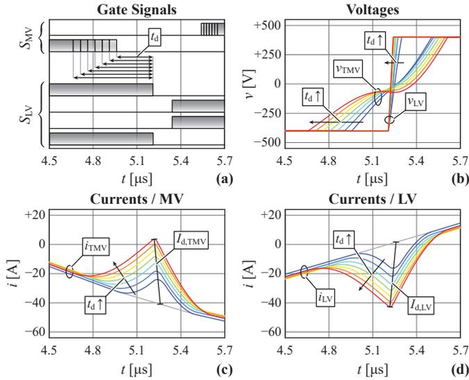
Fig. 11. Simulated ZVS transition with MCS-ZVS modulation for different time delays ( $f_s = 48\text{kHz}$ ,  $P = 25\text{kW}$ ,  $t_d \in [+250, +550]\text{ns}$ , and power flow from the LV to the MV-side). (a) Applied gate signals, (b) bridge voltages, (c) LV currents, and (d) MV currents.
