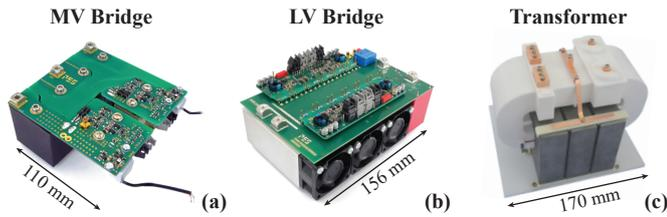
Fig. 15. Considered 25kW SRC-DCX operated at 48kHz between a 7kV and a 400V DC-bus (cf. Fig. 2(a) and Tab. I): (a) MV bridge based on 10kV SiC MOSFETs, (b) LV bridge based on 1200V SiC MOSFETs, and (c) medium-frequency transformer.
