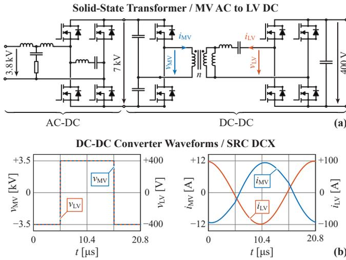
Fig. 1. (a) Considered SST consisting of an AC-DC converter and an isolated DC-DC converter. (b) Schematic view of the current and voltage waveforms of the SRC operated as DCX.
