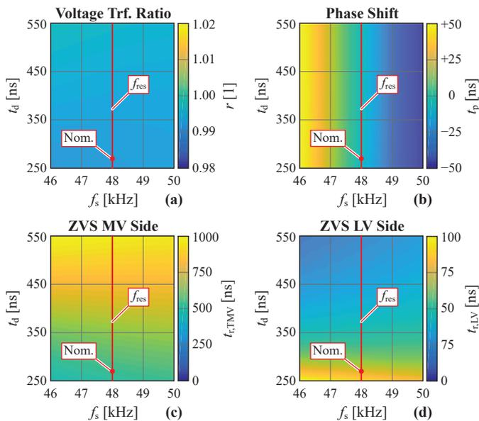
Fig. 13. Simulated (a) voltage transfer ratio (cf. (5)), (b) phase shift between the bridge voltages (computed between the first Fourier harmonics), (c) MV ZVS switching durations, and (d) LV ZVS switching durations. The SRC-DCX is operated with MCS-ZVS modulation ( $P = 25$  kW and power flow from the LV to the MV-side). Different time delays ( $t_d$ ) and operating frequencies ( $f_s$ ) are considered. The nominal operating point ( $f_s = 48$  kHz,  $t_d = 270$  ns) is indicated.
