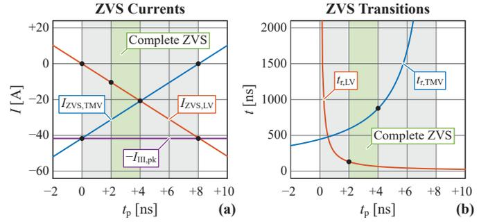
Fig. 10. Calculated (a) ZVS currents and (b) ZVS transition durations obtained for the SRC-DCX operated with MCS-ZVS modulation ( $f_s = 48\text{kHz}$ ,  $t_p \in [-2, +10]\text{ns}$ ). Complete ZVS is calculated as achievable within a reasonable dead time for  $I_{ZVS, LV} < -10\text{A}$  and  $I_{ZVS, TMV} < -20\text{A}$ . For the calculation of the currents, the semiconductor output capacitances of the bridges are neglected and ideal instantaneous switching transitions are considered.
