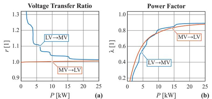
Fig. 6. (a) Voltage transfer ratio (cf. (5)) and (b) power factor (cf. (6)). The SRC-DCX is operated with a passive rectifier bridge ( $f_s = 48\text{kHz}$ ) at different load conditions and for both power flow directions.
