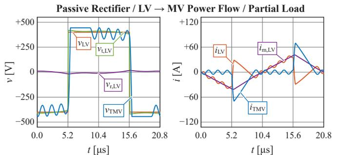
Fig. 7. Simulated voltages and currents at partial load with a passive rectifier bridge ( $f_s = 48\text{kHz}$  and  $P = 5\text{kW}$ ). The power flow is directed from the LV bridge (active) to the MV bridge (passive).
