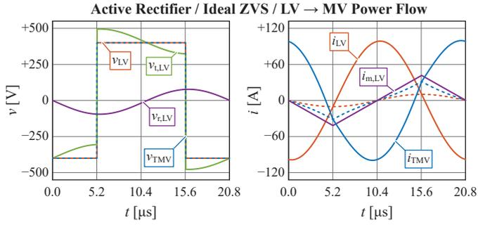
Fig. 9. Calculated voltages and currents with MCS-ZVS modulation ( $f_s = 48\text{kHz}$ ,  $t_p = 2\text{ns}$ ,  $P = 25\text{kW}$ , and power flow from the LV to the MV-side). The reactive currents ( $i_{TMV} - i_{i, TMV}$  and  $i_{LV} - i_{i, LV}$ ) are indicated with dashed lines for both bridges. For the calculation, the semiconductor output capacitances of the bridges are neglected and perfect switching transitions are considered.
