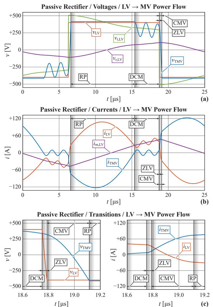
Fig. 3. Simulated (a) voltages and (b) currents with an active LV bridge and a passive MV rectifier ( $f_s = 40$  kHz,  $P = 25$  kW, and power flow from the LV to the MV-side). (c) Voltages and currents during the ZVS switching transition. The different operating modes (time intervals) occurring in one switching cycle are indicated.
