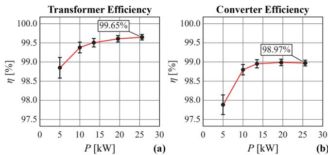
Fig. 17. (a) Measured efficiency of the transformer and (b) DC-DC converter with the corresponding measurement tolerance. More details on the measurement of the losses can be found in [6].
