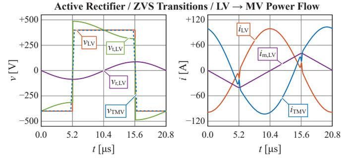
Fig. 12. Simulated voltages and currents with MCS-ZVS modulation ( $f_s = 48\text{kHz}$ ,  $t_d = 270\text{ns}$ , and  $P = 25\text{kW}$ , and power flow from the LV to the MV-side). The reactive currents (circulating current and magnetizing current) are almost exclusively flowing in the MV bridge (cf. (27)) and the LV bridge is switched with the current distortion (cf. (38)).
