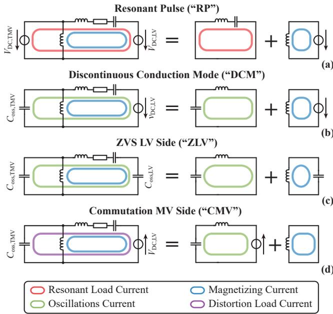
Fig. 4. Equivalent circuits during the different operating modes (time intervals occurring in one switching cycle, cf. Fig. 3): (a) Resonant Pulse (“RP”), (b) Discontinuous Conduction Mode (“DCM”), (c) ZVS LV-Side (“ZLV”), and (d) Commutation MV-Side (“CMV”).
