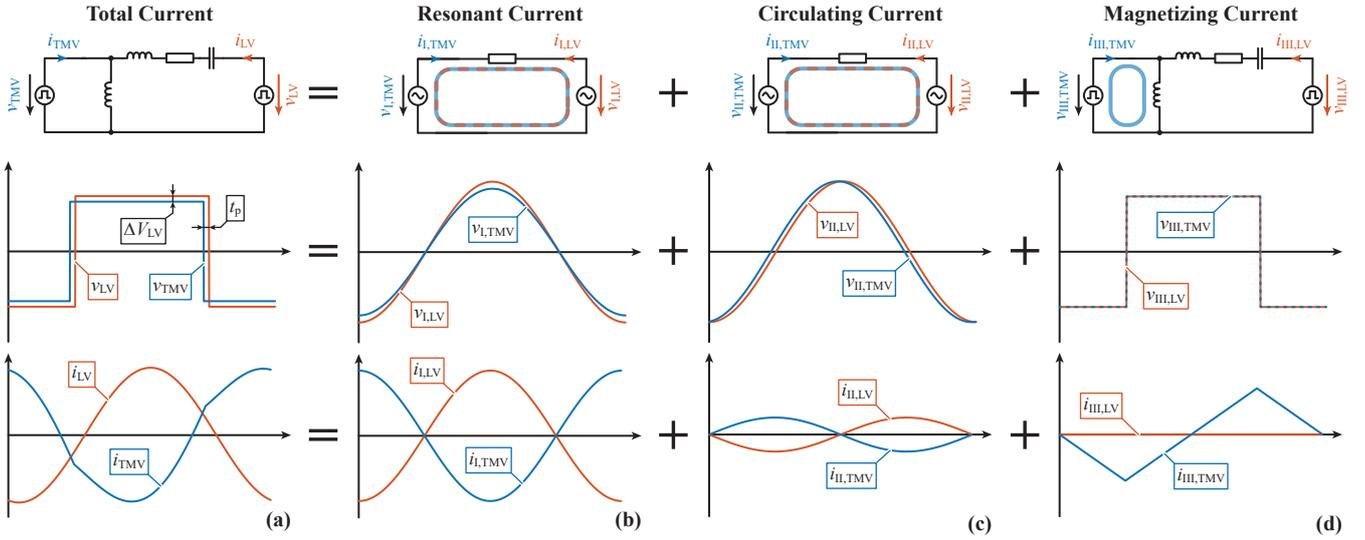
Fig. 8. (a) Equivalent circuit of the SRC-DCX (with a schematic view of the waveforms) operated with MCS-ZVS modulation (phase shifted PWM voltages with 50% duty cycle). The total current in the SRC-DCX can be decomposed into three parts: (b) the resonant current, (c) the circulating current, and (d) the magnetizing current. A power flow from the LV to the MV-side is considered.
