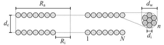
**Figure 5:** Schematic drawing of the cross section of the circular IPT coils including the geometry parameters of the parameter sweep. The geometry is defined by the inside and outside coil radius  $R_i$  and  $R_a$ , and the coil separation distance  $d_c$ . The litz-wire used for the windings has a diameter  $d_w$  and is composed of  $n$  strands with a diameter of  $d_i$ .
