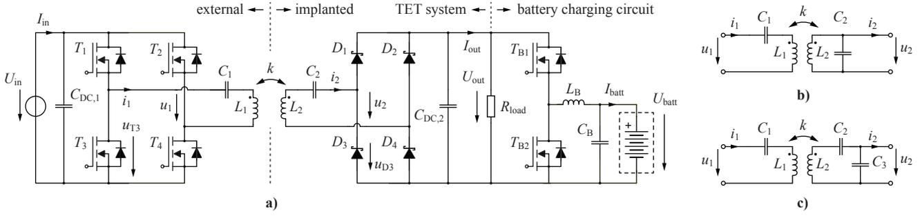
**Figure 2:** a) Proposed series-series resonant topology of the TET system and the backup battery charging controller. The motor inverter and the blood pump is modeled as a single equivalent load resistor. b)-c) show two other compensation methods for the resonant circuit.
