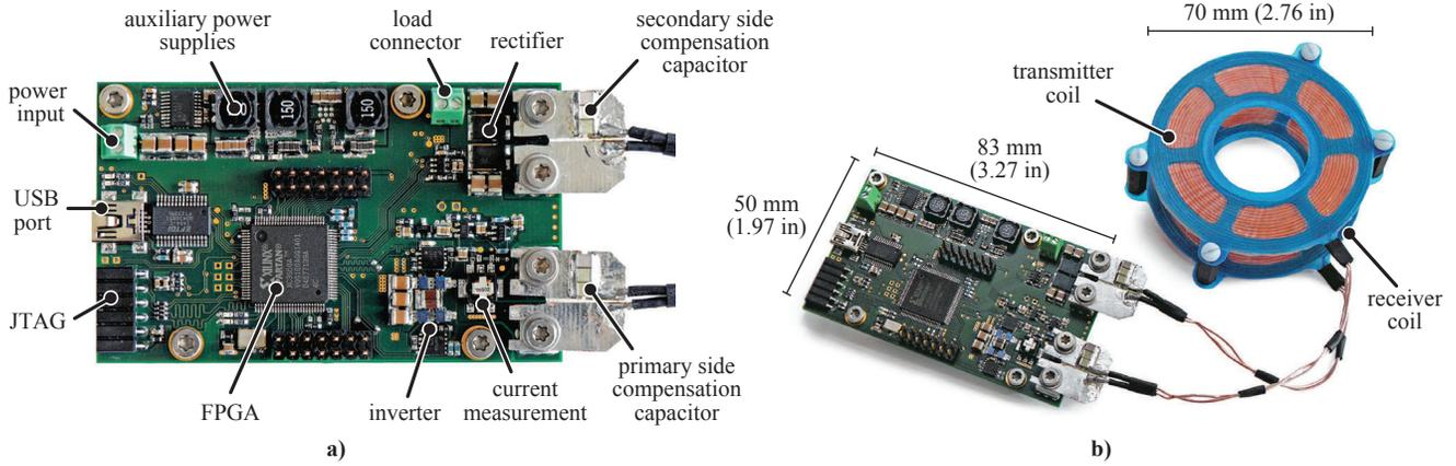
**Figure 8:** Photograph of the converter board and the TET system assembly including the prototype energy transmission coils.
