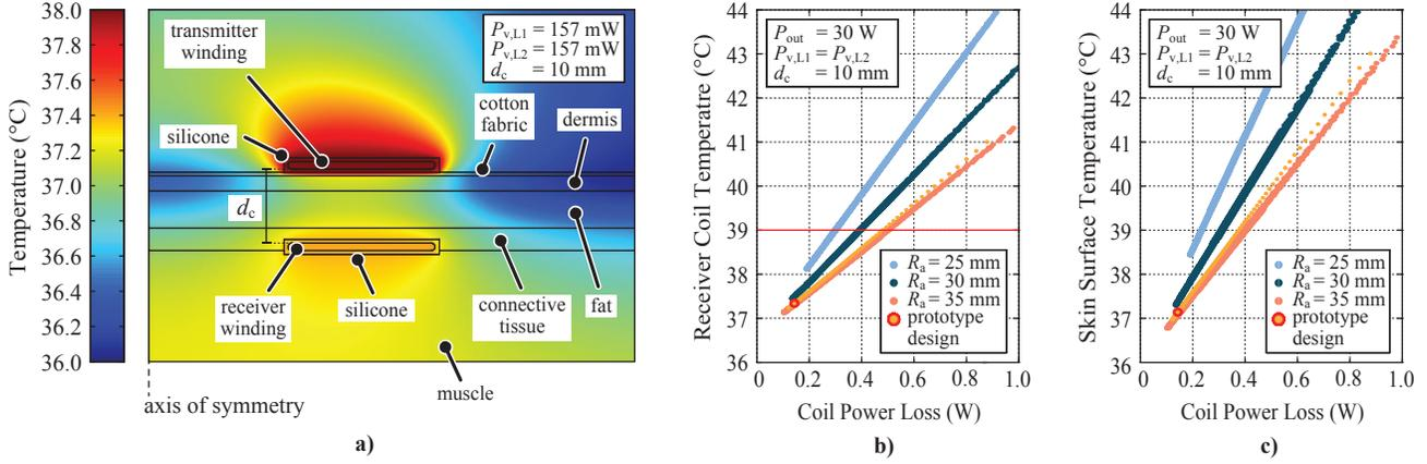
**Figure 6:** a) Structure of the two dimensional thermal model and the spatial temperature distribution of the prototype coils operated at the maximum output power and the minimum coil separation distance, where the primary and secondary side coil losses are equal. b)-c) Simulation results of the maximum surface temperature of the receiver coil and the skin for the coil designs found in **Section IV** under the same operating conditions.
