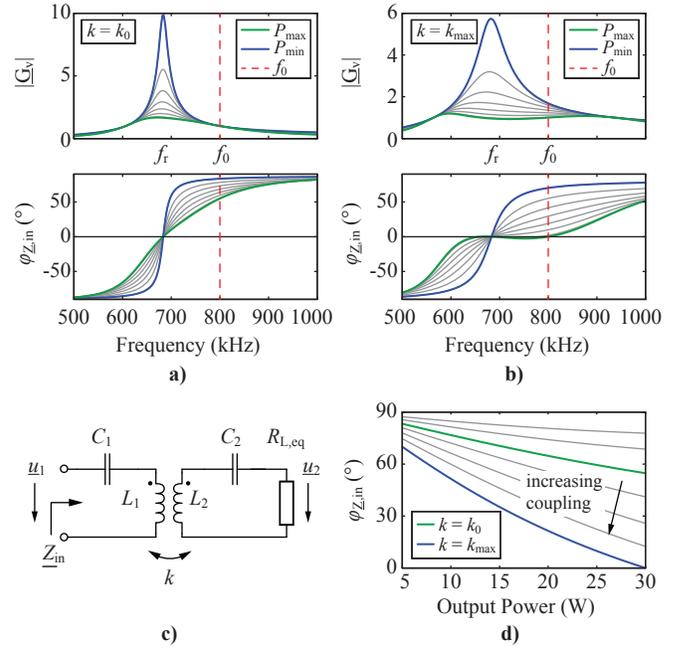
**Figure 3:** a)-b) Voltage transfer characteristics and phase angle of the input impedance of the considered series-series resonant energy transmission system, designed for an operation at 800 kHz, under variable loading conditions. c) Equivalent circuit of the resonant system used for the theoretical analysis. d) Phase angle of the input impedance at variable output power and coupling.
