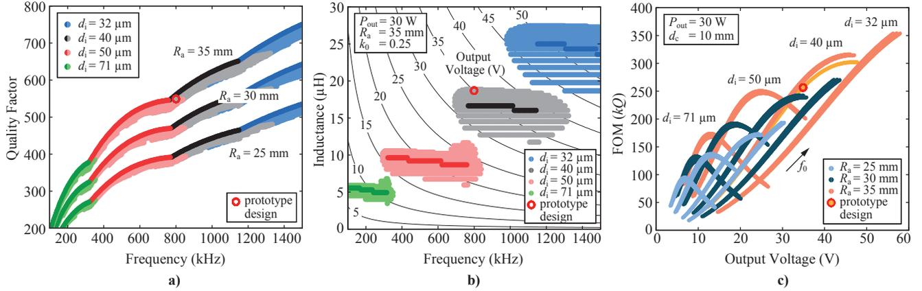
**Figure 4:** a) Designs with the maximum quality factor and designs that exhibit a high quality factor within 5% of the maximum value for different coil diameters. b) Load matching plane defined by (7) for the same coil designs with an outside coil radius of 35 mm (1.38 in). c) Coil designs with the largest Figure-of-Merit  $FOM = kQ$  at minimum coil separation distance with respect to the TET system output voltage.
