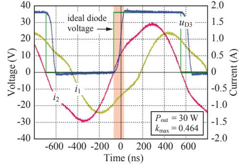
**Figure 10:** Deviation of the measured rectifier diode  $u_{D3}$  from the ideal switching waveform, as well as the primary and secondary side currents  $i_1$  and  $i_2$ . The red shading highlights the time interval, where the parasitic capacitances of the rectifier diodes must be either charged or discharged in order to commutate the current to the active branch of the rectifier.
