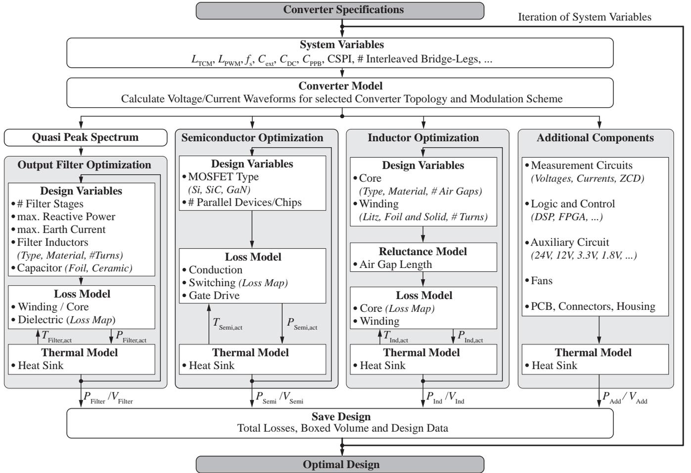
**Fig. 10:** Flow chart of the  $\eta\rho$ -Pareto optimization procedure.
