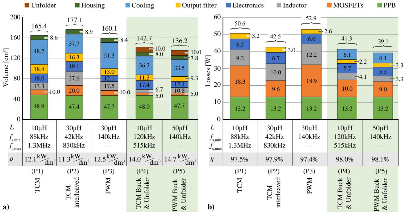
**Fig. 11: a)** Volume distribution and **b)** loss distribution of all designs achieving the respective highest power density (P1-P5).
