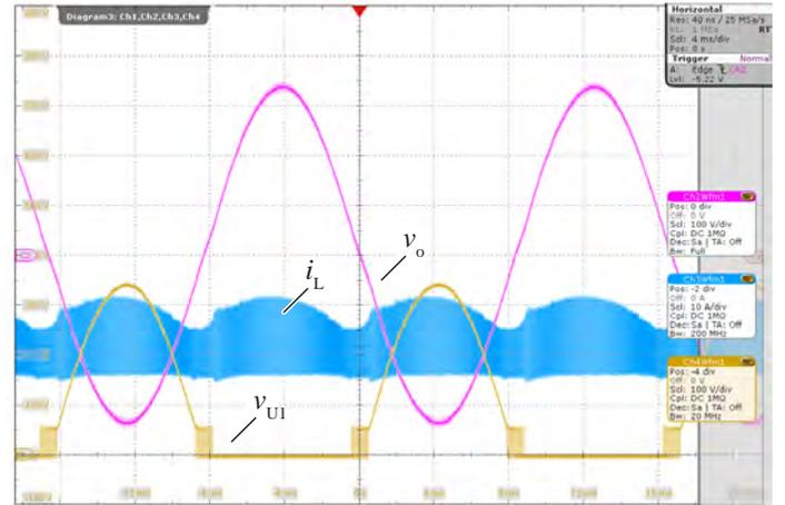
**Fig. 9:** Measured waveforms of the proposed modulation strategy for the DC-|AC| Buck Converter & Unfolder of **Fig.7** at an output power of 1 kW. Inductor current  $i_L$  (10 A/div), bridge-leg voltage  $v_{U1}$  (100 V/div) and output voltage  $v_o$  (100 V/div).
