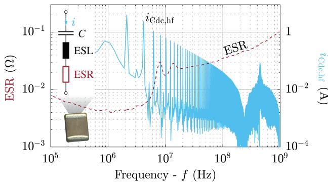
**Fig. 8:** Fourier transform of the simulated  $i_{\text{Cdc,hf}}$  (solid) and nominal ESR of  $C_{\text{dc,hf}}$  [19] (dashed) considered to calculate the losses occurring in  $C_{\text{dc,hf}}$  during switching operation.
