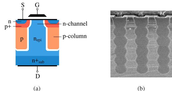
**Fig. 1:** Cross-section of a SJ Si MOSFET highlighting (a) the different doping concentrations and the characteristic 3D structure of p- and n-columns and (b) the inhomogeneity of the doping profiles as a result of the multi-epitaxy technology and subsequent implantation of p-dopants.
