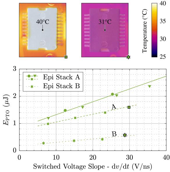
**Fig. 20:**  $E_{P\text{TO}}$  as function of  $\frac{dv_{\text{PTO}}}{dt}$  obtained with different  $I_{\text{sw}}$  (5 A...20 A) for  $V_{\text{dc}} = 400$  V.  $E_{P\text{TO},B}$  (dotted) is more than 70 % lower than  $E_{P\text{TO},A}$  (dashed). Additionally, thermal images of the two analyzed PTO DUT featuring different epitaxial stacks: B (right) experiences only one tenth of the temperature increase of A (left).
