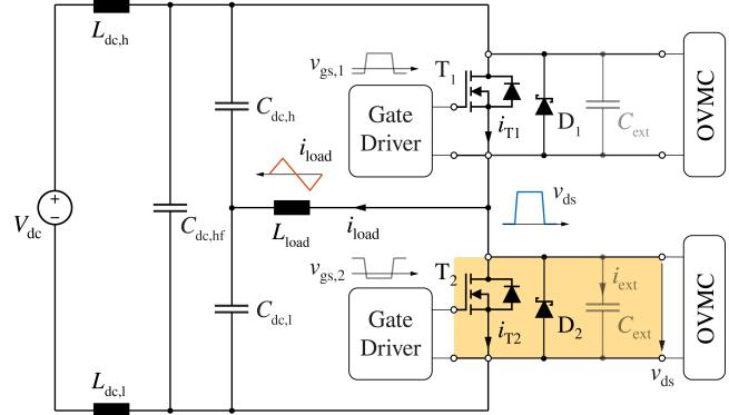
**Fig. 2:** Schematic of the realized soft-switching loss measurement setup consisting of the half-bridge formed by the two DUT T<sub>1</sub> and T<sub>2</sub>. With the considered modulation scheme ( $v_{gs,1}$  and  $v_{gs,2}$ ), the illustrated waveforms of  $v_{ds}$  and  $i_{load}$  are obtained.
