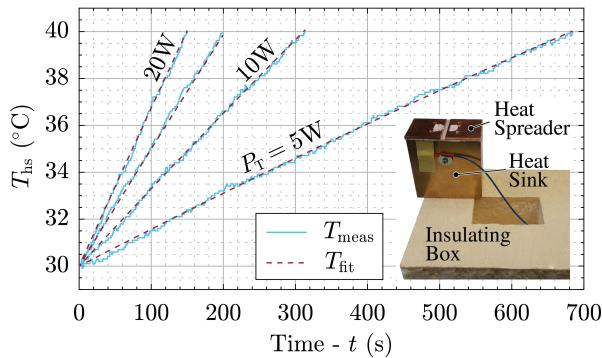
**Fig. 6:**  $T_{\text{meas}}$  (solid) and  $T_{\text{fit}}$  (dashed) for different  $P_T$ . The agreement of the model (see Fig. 5 (a) and Table III) with the experimental data is satisfactory.
