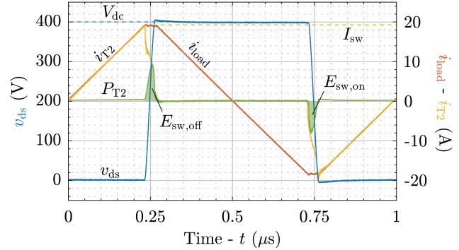
**Fig. 4:** Main waveforms characterizing the half-bridge of **Fig. 2** in soft-switching operation, i.e.  $v_{\text{ds}}$ ,  $i_{\text{load}}$ ,  $i_{T2}$  and  $P_{T2}$  for one switching period ( $f_{\text{sw}} = 1 \text{ MHz}$ ) in case  $V_{\text{dc}} = 400 \text{ V}$  and  $I_{\text{sw}} \approx 20 \text{ A}$ .
