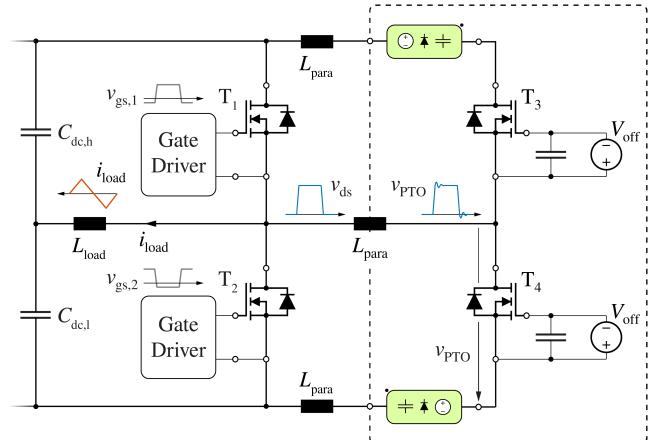
**Fig. 11:** Schematic of the realized measurement setup consisting of the half-bridge formed by the PTO DUT  $T_3$  and  $T_4$  (dashed box) connected in parallel to the switching half-bridge  $T_1-T_2$ .  $T_1$  and  $T_2$  generate high  $dv/dt$  square-wave voltage waveforms across the drain and source terminals of  $T_3$  and  $T_4$ .
