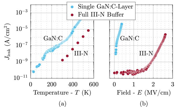
**Fig. 17:** Measured  $J_{leak}$  of a single GaN:C-layer compared to a complete multi-layer III-N buffer as function of (a) temperature and (b) vertical electric field.
