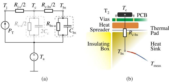
**Fig. 5:** (a) Thermal equivalent circuit of the calorimetric loss measurement setup and (b) vertical stack of the elements forming  $R_{c-hs}$ .
