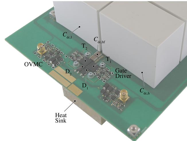
**Fig. 3:** Picture of the realized soft-switching loss measurement setup. The switching half-bridge formed by the two DUT T<sub>1</sub> and T<sub>2</sub>, the anti-parallel diodes D<sub>1</sub> and D<sub>2</sub>, the gate drivers, the OVMCs and the capacitors  $C_{dc,h}$ ,  $C_{dc,l}$  and  $C_{dc,hf}$  are highlighted.
