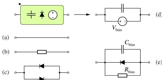
**Fig. 13:** Different solutions to interconnect the half-bridges; (d) is preferred since properly adjusting  $V_{\text{bias}}$ , the reverse conduction of both PTO DUT is prevented.
