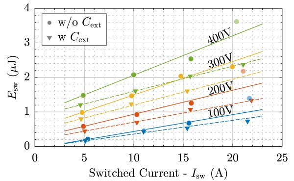
**Fig. 9:**  $E_{\text{sw}}$  as function of  $I_{\text{sw}}$  (5 A... 20 A) for different  $V_{\text{dc}}$  (100 V... 400 V).  $E_{\text{sw}}$  without (dots) and with (triangles)  $C_{\text{ext}}$  are compared.
