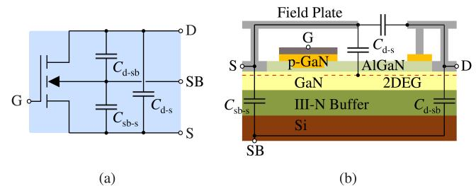
**Fig. 16:** (a) Equivalent circuit and (b) cross-section of the DUT illustrating the main structural components determining the parasitics capacitors  $C_{\text{d-s}}$ ,  $C_{\text{sb-s}}$  and  $C_{\text{d-sb}}$ .
