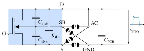
**Fig. 18:** Equivalent circuit of the DUT and schematic representation of the jumpers allowing to connect the source and substrate terminals of the low-side SS DUT to either AC or GND.
