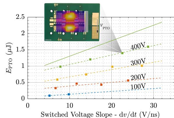
**Fig. 15:**  $E_{\text{PTO}}$  as function of  $\text{dv}_{\text{PTO}}/\text{dt}$  obtained with different  $I_{\text{sw}}$  (5 A... 20 A) for different  $V_{\text{dc}}$  (100 V... 400 V).  $E_{\text{PTO}}$  (dashed) constitutes from 70 % to 90 % of  $E_{\text{sw}}$  (solid) in the case of  $V_{\text{dc}} = 400 \text{ V}$ .
