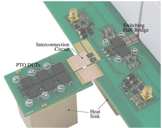
**Fig. 12:** Picture of the realized measurement setup for the PTO DUT. On the right hand-side PCB, the switching half-bridge is highlighted. On the left hand-side PCB, the half-bridge formed by the PTO DUT separated by the interconnection circuit from the switching half-bridge is visible (see **Fig. 13**).
