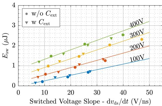
**Fig. 10:**  $E_{sw}$  as function of  $dv_{ds}/dt$  obtained with different  $I_{sw}$  (5 A... 20 A) for different  $V_{dc}$  (100 V... 400 V).  $E_{sw}$  without (dots) and with (triangles)  $C_{ext}$  follow the same interpolation lines (solid).
