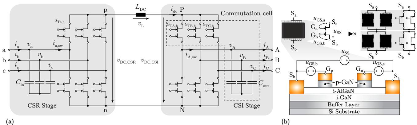
**Fig. 1.** (a) AC-AC CSC with AC-side filter capacitors (DM and CM EMI filter stages not shown). (b) Realization of a bidirectional switch (BDS) with four discrete unipolar GaN devices to achieve equal total on-state resistance as for a single unipolar device, and alternative realization as a dual-gate GaN monolithic BDS (M-BDS) with a shared drain-gate region for blocking either voltage polarity and accordingly substantially lower chip area.
