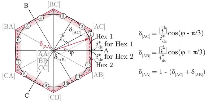
**Fig. 2.** Exemplary space vector diagram for a CSI stage with exemplary equations of the dwell times needed to synthesize the exemplary reference current vector  $\vec{i}^*$ . In case of 2/3-PWM, the shaping of the DC-link current  $i_{dc}$  corresponds to a continuous scaling of the hexagon spanned by the space vectors such that its perimeter always coincides with the trajectory of the reference current vector  $\vec{i}^*$ .
