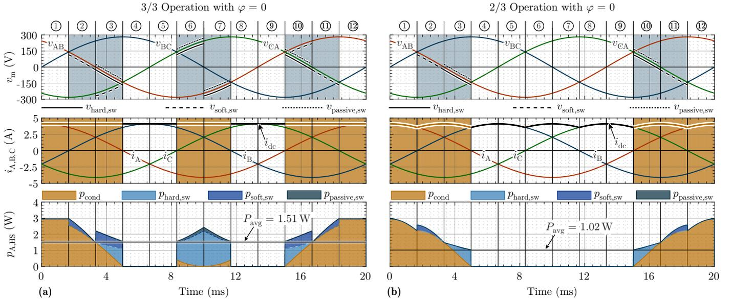
**Fig. 7.** Loss components of  $S_{TA,h}$ , i.e., the high-side transistor of the CSI's phase A, over a fundamental period for (a) 3/3-PWM and (b) 2/3-PWM for an exemplary operating point with  $V_m = 200$  V,  $I_m = 4$  A, and a switching frequency of 100 kHz. Note especially the absence of switching losses in sectors 6 and 7 in case of 2/3-PWM, i.e., in the region with the highest phase current magnitude and also the highest switched line-to-line voltage in case of 3/3-PWM.
