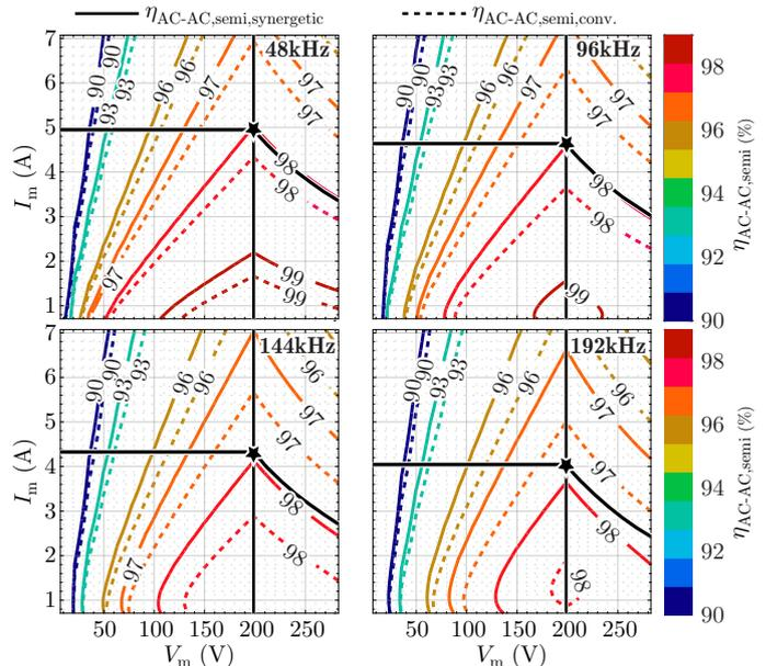
**Fig. 9.** Semiconductor AC-AC efficiency characteristics of a CSC motor drive employing the novel GaN M-BDSs and operating with or without the proposed synergetic control at different switching frequencies. The thick black lines indicate the output rms current limits that ensure  $T_j = 100$  °C and which are very similar for both cases, i.e., conventional control and the proposed synergetic control, because always the stage operating with 3/3-PWM limits the allowable current (see **Fig. 8**).
