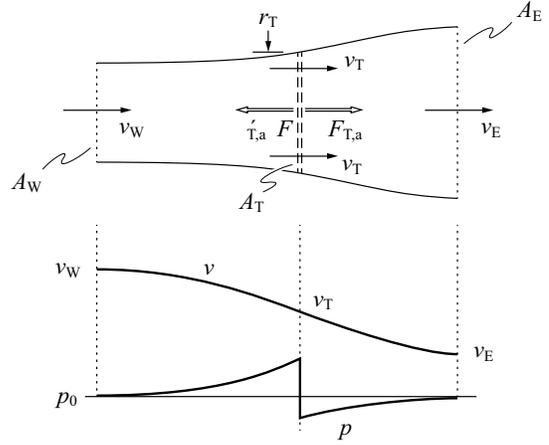
Fig. 38. Setup considered for the derivation of Betz' Law (airflow tube with turbine replaced by actuator disk); wind speed and pressure profile.
