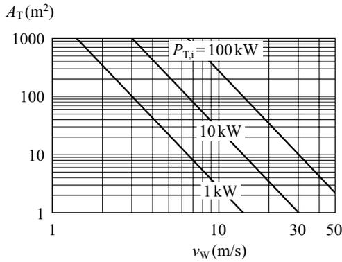
Fig. 1. Dependency of the maximum output power  $P_{T,i}$  of a wind turbine on the area  $A_T$  swept by the rotor blades and the wind speed  $v_W$  [cf. (1) and (71), parameter  $c_p = c_{p,i} = 0.59$ ].
