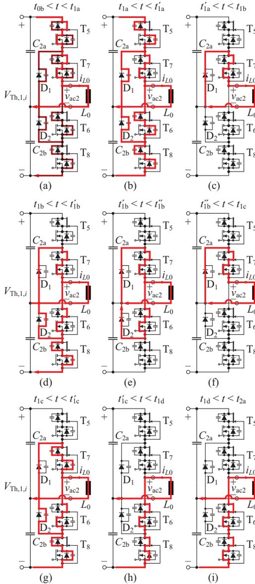
Fig. 20. Transient conduction paths during  $t_{1a} < t < t_{1d}$ , cf. Fig. 19(b). (a)–(f)  $v_{ac2}$  is switched from  $V_{Th,1,i}/2$  to 0. (g)–(i)  $v_{ac2}$  is switched from 0 to  $-V_{Th,1,i}/2$  (Figs. from [32]).
