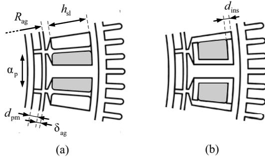
Fig. 12. Definition of machine dimensions. (a) LV machine. (b) MV machine with additional insulation. The windings around a stator tooth are highlighted in gray.
