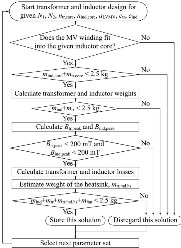
Fig. 26. Flowchart showing the procedure employed to design the HF transformer and the inductor of the DAB. With this design procedure, the results shown in Fig. 27 are calculated.
