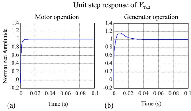
Fig. 36. Unit step response of closed-loop reference tracking transfer function  $G_{vTh2,cl}$  for (a) motor operation and (b) generator operation.
