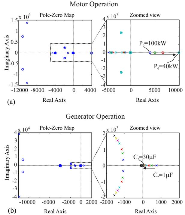
Fig. 33. Pole-zero map of the open-loop transfer function  $G_{vTh2,Ruout}$  for (a) motor operation; the RHP zero moves farther to the right for lower output power  $P_0$ . (b) Generator operation; the zoomed view is shown that the unstable RHP pole moves toward the origin for higher values of  $C_2$ .
