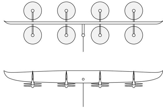
Fig. 3. Conceptual drawing of aerofoil and turbines of a 100 kW AWT system of Joby Energy [3]; length / width: 11 m / 1 m.
