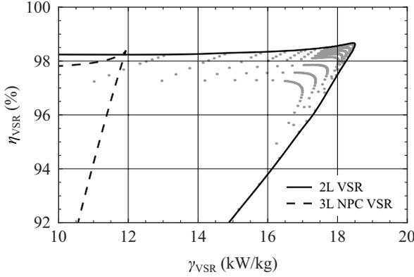
Fig. 16. Efficiency versus power-to-weight ratio of the 2L VSR and the 3L VSR. With the 2L VSR, a significantly higher power-to-weight ratio at a similar maximum efficiency is achievable, compared with the 3L VSR.
