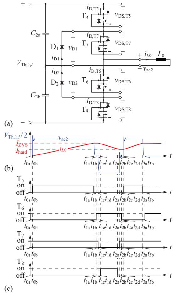
Fig. 19. (a) Switching loss measurement setup (NPC converter). (b) Employed measurement waveforms: (almost) ZVS during  $t_{1a} < t < t_{1d}$ , hard switching during  $t_{2a} < t < t_{2d}$ . (c) Respective gate signals of  $T_5$ ,  $T_6$ ,  $T_7$ , and  $T_8$  (Figs. from [32]). The dead time used to avoid a shoot through is 200 ns.
