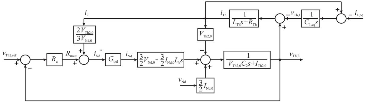
Fig. 34. Control block diagram.
