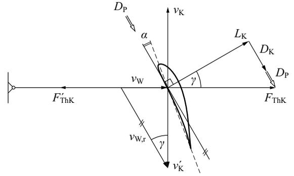
Fig. 41. Velocity components and forces acting on the power kite of an AWT (turbines not shown, cf. Fig. 42).
