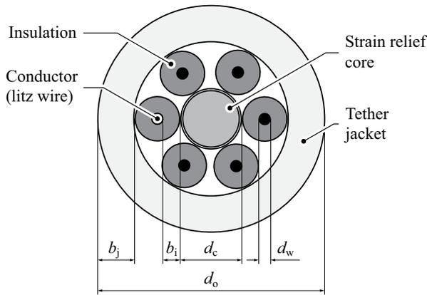
Fig. 7. Cross-section of the designed tether, showing its assembly with a center-aligned strain relief core, six litz wire conductors with insulation arranged around the core, and the tether protection jacket. An additional insulation layer could be wrapped around all conductors.
