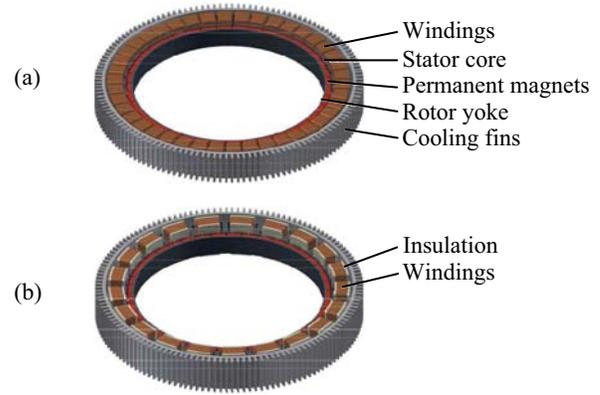
Fig. 10. CAD drawing. (a) LV machine. (b) MV machine with extra insulation.
