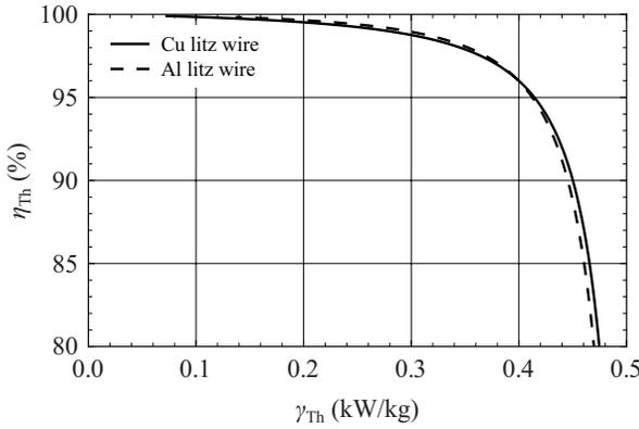
Fig. 9. Efficiency versus power-to-weight ratio of the tether for copper (Cu) and aluminum (Al) litz wire conductors at a tether dc-voltage of 8 kV.
