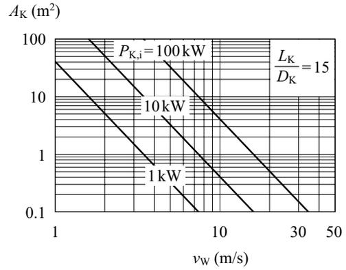
Fig. 43. Dependency of the power kite output power on the effective air velocity  $v_{W,r}$  and the kite area  $A_K$  under the assumption of optimal selection of  $D_P$ , i.e.,  $D_P = D_{P,i} = 1/2 D_K$ ; cf. (95).
