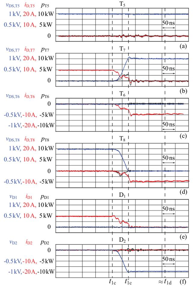
Fig. 23. Measured instantaneous currents and voltages of the switches and diodes of the NPC converter depicted in Fig. 19(a) for  $v_{ac2}$  being switched from 0 to  $-V_{Th,1,i}/2$ ;  $V_{Th,1,i} = 2$  kV,  $i_{L0}(t_{1c}) = I_{ZVS} = 10$  A (Figs. from [32]). During  $t_{1c} < t < t'_{1c}$  the energy stored in the output capacitance of  $T_8$  is transferred to that of  $T_7$ .
