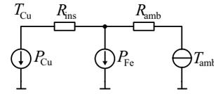
Fig. 11. Thermal equivalent circuit of the machine with resistive losses  $P_{Cu}$  and iron losses  $P_{Fe}$ , and thermal resistance of the winding insulation  $R_{ins}$  and thermal resistance to the ambient  $R_{amb}$ .
