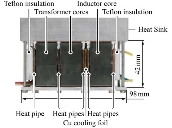
Fig. 28. Picture of the realized HF transformer and the inductor (Fig. from [32]).
