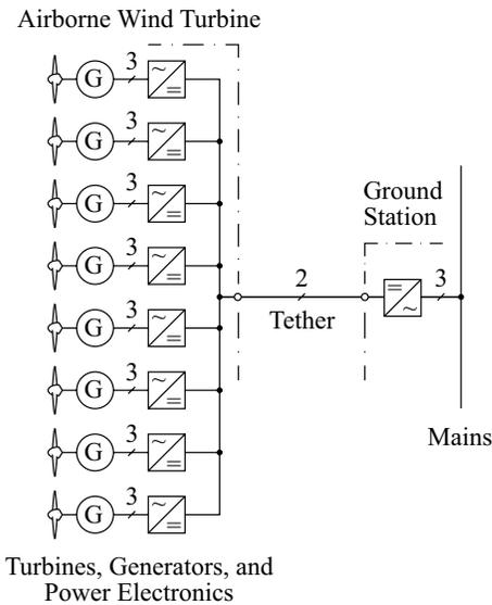
Fig. 5. AWT basic electric system structure.
