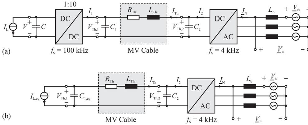
Fig. 32. (a) Equivalent circuit of the AWT power electronic system. (b) Simplified equivalent circuit assuming that the dc-dc converter behaves like an ideal transformer [cf. (39)–(41)].
