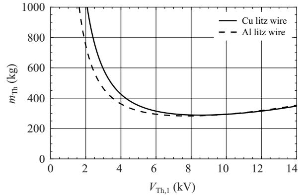
Fig. 8. Tether mass versus tether dc-voltage for copper (Cu) and aluminum (Al) litz wire conductors for a fixed tether efficiency  $\eta_{Th} = 98.5\%$  (1.5 kW conduction losses at a power input of 100 kW).
