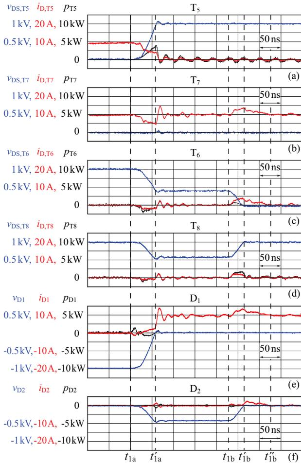
Fig. 22. Measured instantaneous currents and voltages of the switches and diodes of the NPC converter depicted in Fig. 19(a) for  $v_{ac2}$  being switched from  $V_{Th,1,i}/2$  to 0;  $V_{Th,1,i} = 2$  kV,  $i_{L0}(t_{1a}) = I_{ZVS} = 10$  A (Figs. from [32]). During  $t_{1b} < t < t'_{1b}$  the switch  $T_6$  generates turn-on losses since its effective output capacitance has not been completely discharged during  $t_{1a} < t < t'_{1a}$ .
