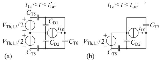
Fig. 21. (a) Simplified equivalent circuit of the NPC converter during  $t_{1a} < t < t'_{1a}$ . (b) Simplified equivalent circuit during  $t_{1c} < t < t'_{1c}$  (Figs. from [32]).
