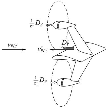
Fig. 42. Schematic representation of an AWT section (power kite wing carrying wind turbines, cf. Fig. 2).
