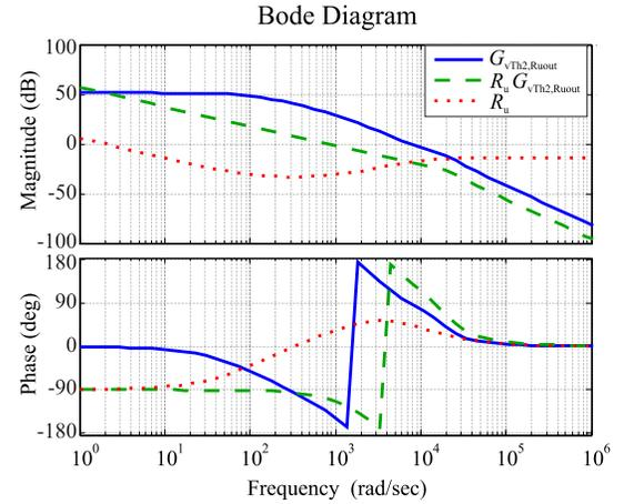
Fig. 35. Bode plot of plant  $G_{vTh2,Ruout}$ , controller  $R_u$  and their open-loop interconnection  $R_u G_{vTh2,Ruout}$  for motor operation  $P_0 = 100$  kW.
