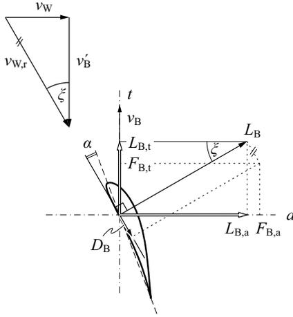
Fig. 40. Velocity components and forces acting on the blade of a CWT.
