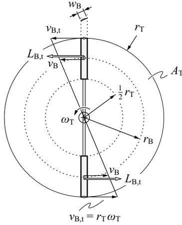
Fig. 39. Turbine swept area and blade area.
