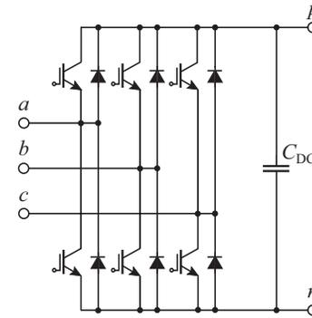
Fig. 14. Circuit topology of the two-level voltage source rectifier (2L VSR).
