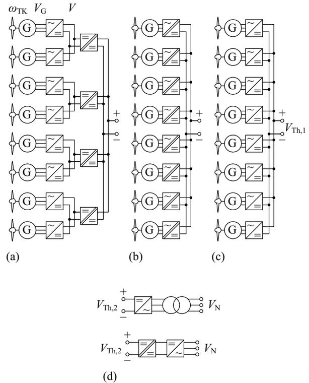
Fig. 6. Selection of possible concepts of AWT power electronics. (a) and (b) LV generators. (c) MV generators. (d) Possible structures of the ground station power electronics and connection to the three-phase mains.
