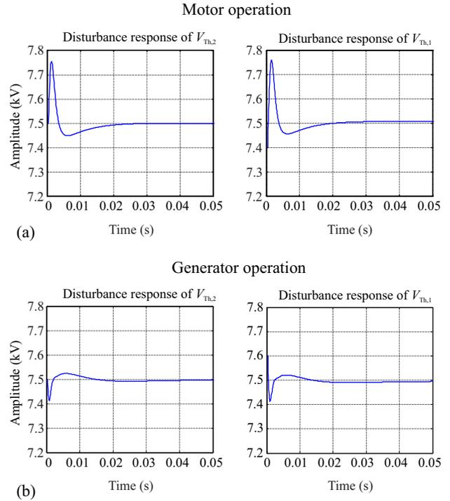
Fig. 37. (a) Response of  $V_{Th,2}$  and  $V_{Th,1}$  on a step in  $i_{L,eq}$  from 13.3 A to 0 A corresponding to a step change of  $P = 100$  kW to  $P = 0$  kW in motor operation. (b) Response of  $V_{Th,2}$  and  $V_{Th,1}$  on a step in  $i_{L,eq}$  from  $-13.3$  A to 0 A corresponding to a step change of  $P = -100$  kW to  $P = 0$  kW in generator operation.
