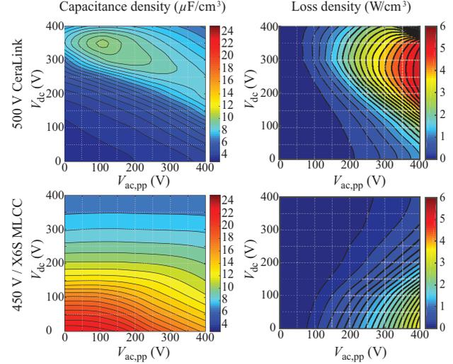
Fig. 22. Contour plot of capacitance density and loss density of a 500 V CeraLink and 450 V class II/X6S capacitor technology with respect to DC bias  $V_{dc}$  and 120 Hz AC excitation  $V_{ac,pp}$  at 60 °C operating temperature.
