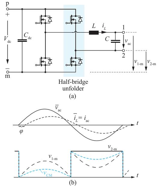
Fig. 12. (a) Half-bridge unfold based inverter topology resembling an H-bridge inverter with asymmetrical bridge-leg filter configuration (only HF bridge-leg is equipped with filter inductor). (b) Characteristic waveforms and resulting low-frequency CM voltage.
