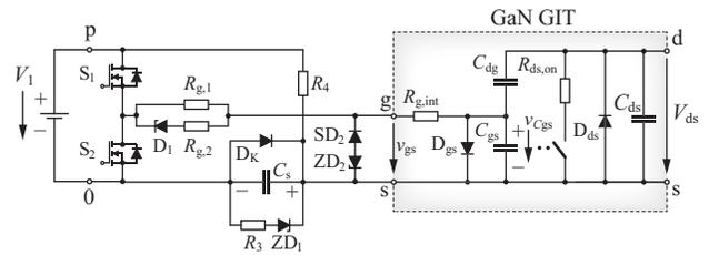
Fig. 3. Proposed improved GaN GIT gate drive circuit [10], [11] to guarantee a reliable gate drive operation with consistent performance regardless of duty-cycle and switching frequency.
