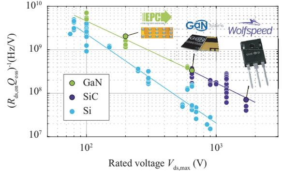
Fig. 2.  $\text{FOM} = 1/(R_{\text{ds,on}}Q_{\text{oss}})$  for the majority of commercially available Si,  $R_{\text{ds,on}}Q_{\text{oss}}$  SiC and GaN power semiconductors in dependency of the rated blocking voltage [7].
