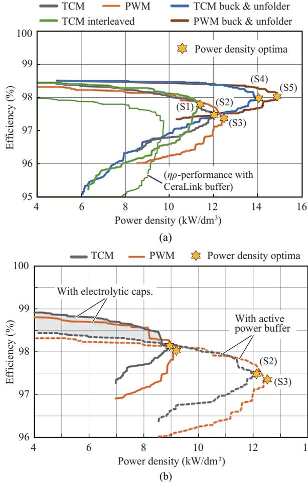
Fig. 18. (a) Computed  $\eta\rho$ -performance of the H-bridge inverter and DC/AC buck-stage with AC/AC H-bridge unfold inverter concept including the active power buffer for different operating modes (TCM/PWM) and with/without interleaving of bridge-legs. (b) Impact of employing the active power buffer on the overall  $\eta\rho$ -performance in comparison to a passive power buffer using electrolytic capacitors.
