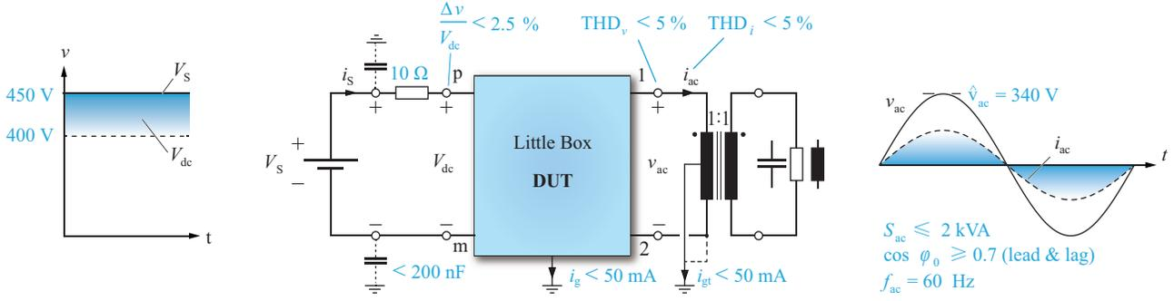
Fig. 1. Google Little Box Challenge test configuration with specified 10 Ω input resistor and 1:1 isolation transformer at the output.
