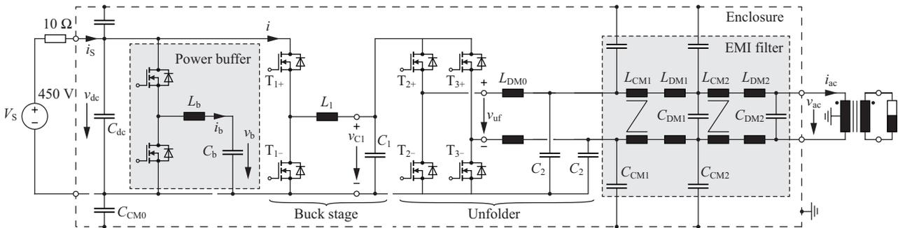
Fig. 17. DC/|AC| buck-stage and |AC|/AC H-bridge unfold inverter with buck-type PCI power buffer and 2-stage EMI filter. The H-bridge based unfold is equipped with DC-link referenced output filter and is temporarily operated with HF PWM around the ZCs of the AC voltage (cf., Section III-C2). The inverter is embedded in the test setup according to the GLBC specifications with split-winding grounding scheme of the isolation transformer.
