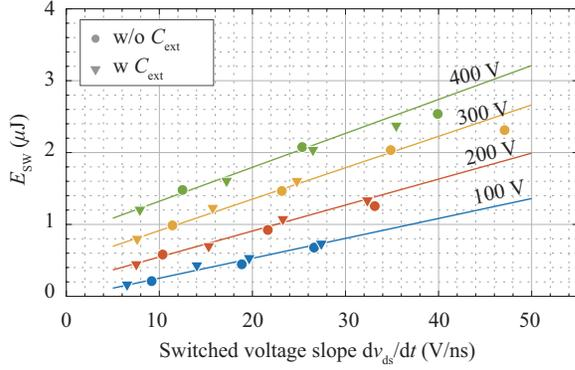
Fig. 20.  $E_{sw}$  reported in [12] as function of  $dv_{ds}/dt$  obtained for several switched currents  $I_{sw}$  (5A,...,20 A) for different  $V_{DC}$  voltage levels (100 V,...,400 V).  $E_{sw}$  without (dots) and with (triangles) added capacitance  $C_{ext} = 100$  pF are well aligned.
