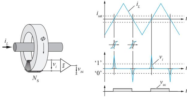
Fig. 5. Zero crossing detection (ZCD) by means of voltage  $v_i$  induced in the pick-up coil ( $N_s = 10$  turns) when the magnitude of current  $i_L$  falls below the saturation threshold  $i_{sat}$  of the employed magnetic core.
