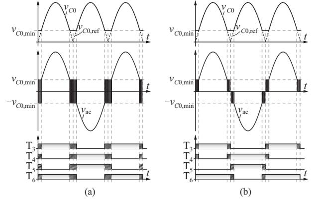
Fig. 11. Clamping of the DC/AC buck-stage output voltage of Fig. 10 (a) to  $v_{C0,min} > 0$  and temporary operation of the unfold H-bridge with (a) bipolar and (b) unipolar HF PWM to prevent distortions around the zero-crossing of the AC voltage.
