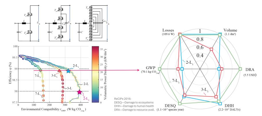
■ Environmental footprint of 2L/3L/7L-designs with  $\eta \approx 99\%$  and max. env. compat.  $\varepsilon_{GWP}$  in W / kg CO<sub>2</sub>eq ■ Same efficiency via different usage of act./pass. components — Different environmental impact profile!
