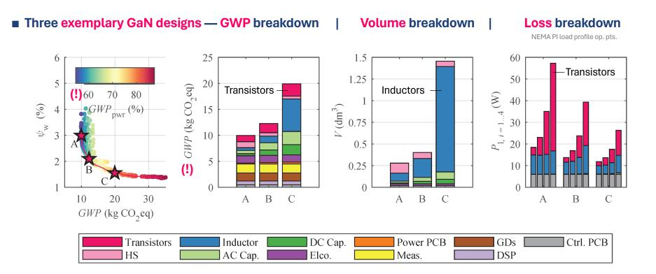
Auxiliary electronics limit min. GWP (!) — Similar: housing, etc. (not considered) — Dep. on rated power!
