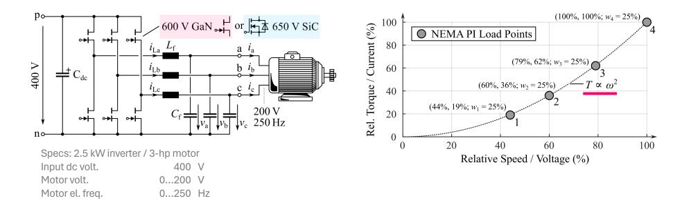
LV VSD inverter w. WBG and dc-bus-referenced LC output filter w. DM & CM attenuation (smooth mot. volt.)
