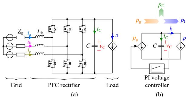
Fig. 1. (a) Schematic drawing of a two-level three-phase boost type PFC rectifier and (b) equivalent circuit illustrating the relations between instantaneous power levels at the DC side. The output load features a controlled-power sink characteristic, i.e.,  $p_l(t)$  tracks a defined time-varying reference.
