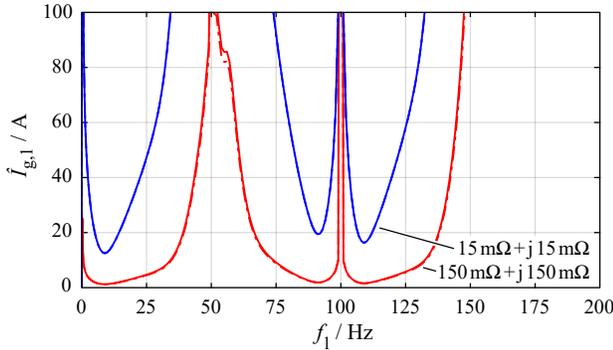
Fig. 5. Maximum acceptable sideband amplitudes of the grid currents to comply with IEC 61000-3-11 (flicker), being evaluated for two different grid impedances. The shown limits are the maximum amplitudes of the sideband currents.
