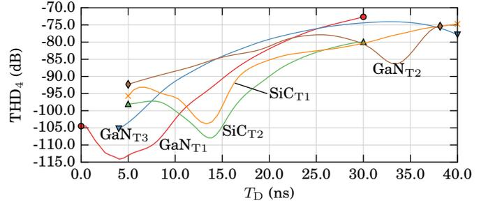
Fig. 11: Influence of the dead time  $T_D$  with different switches in the HB topology.  $f_{PWM} = 100$  kHz,  $f_T = 50$  Hz,  $f_o = 2$  kHz,  $m = 0.75$ ,  $i_o = 3$  A,  $\varphi_o = 0^\circ$ ,  $U_{DC} = 400$  V (150 V with GaN<sub>T2</sub>).
