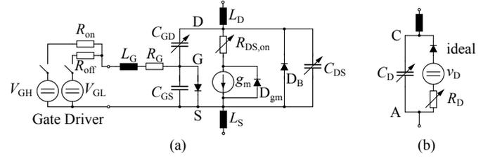
Fig. 5: (a): Electrical transistor and (b): diode model used for the simulations. All parameters are derivable from datasheet specifications.
