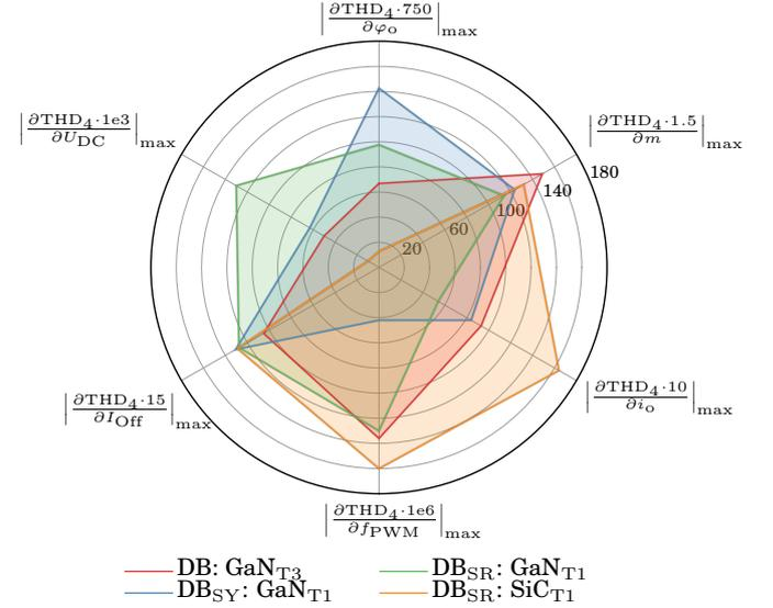
Fig. 14: Maximum of the absolute values of the sensitivities in their respective parameter ranges (cf. Tab. II) for different dual buck topologies.
