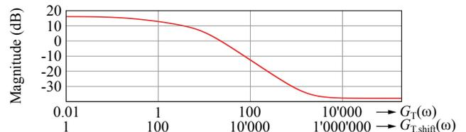
**Fig. 7:** Magnitude plot of an exemplary thermal transfer function and the effect of the frequency shift.  $f_o = 100f_T$
