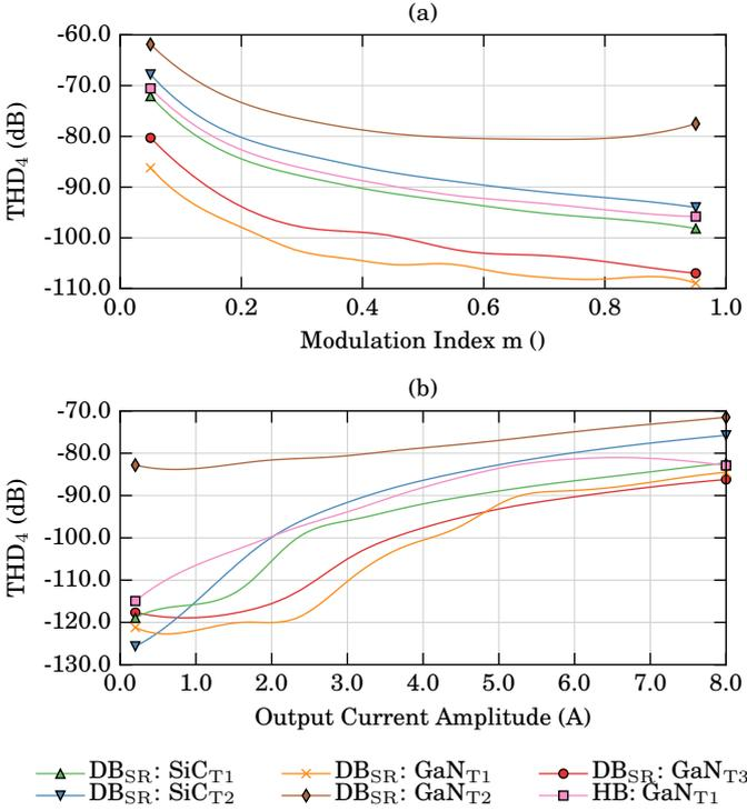
Fig. 10: Comparison of different switch technologies. THD as a function of (a): the modulation index  $m$  and (b): the output current amplitude  $i_o$ .  $f_{PWM} = 100$  kHz,  $f_T = 50$  Hz,  $f_o = 2$  kHz,  $m_{nom} = 0.75$ ,  $i_{o,nom} = 3$  A,  $\varphi_o = 0^\circ$ ,  $T_{D,HB} = 15$  ns,  $T_{D,DBSR} = 20$  ns,  $I_{Off} = 5$  A,  $U_{DC} = 400$  V (150 V with GaN<sub>T2</sub>).
