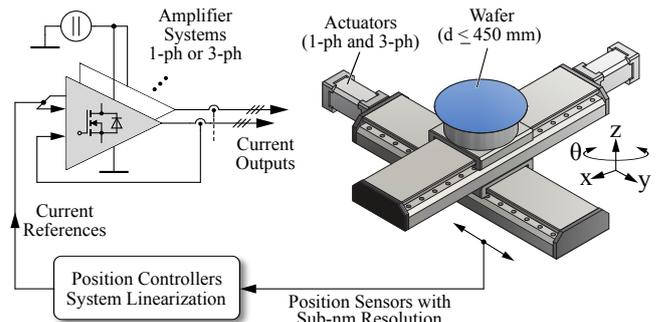
Fig. 1: Wafer positioning system. Different kinds of actuators such as voice coils (1-phase) or permanent magnet motors (3-phase) are driven by precision amplifiers which must provide a high current quality to avoid undesired mechanical movement and to achieve high control dynamics to ensure fast wafer positioning and/or high productivity.
