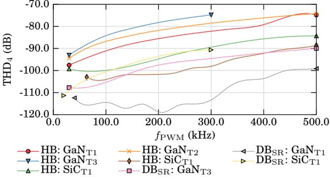
Fig. 13: Influence of the switching frequency  $f_{\text{PWM}}$  with different switches in different HB and DB topologies.  $f_{\text{T}} = 50$  Hz,  $f_{\text{o}} = 2$  kHz,  $m = 0.75$ ,  $i_{\text{o}} = 3$  A,  $\varphi_{\text{o}} = 0^\circ$ ,  $T_{\text{D,HB}} = 15$  ns.
