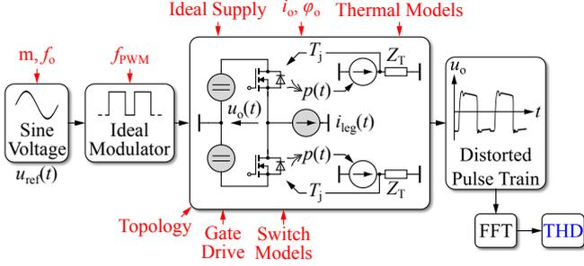
Fig. 3: Simulation setup for the distortion analysis of the switching stage. Different circuit topologies, switch technologies and thermal systems are modeled such that the main nonlinearities are well accounted for. All functional blocks except the switching stage are assumed ideal.
