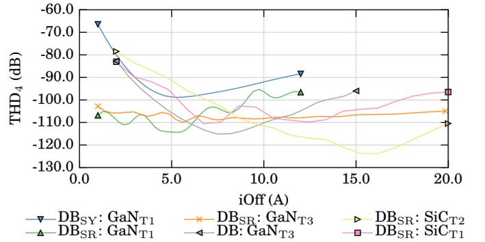
Fig. 12: Influence of the offset current  $I_{Off}$  with different switches in different DB topologies.  $f_{PWM} = 100$  kHz,  $f_T = 50$  Hz,  $f_o = 2$  kHz,  $m = 0.75$ ,  $i_o = 3$  A,  $\varphi_o = 0^\circ$ .
