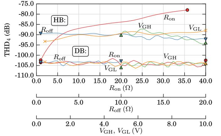
Fig. 8: Sensitivities to the gate driver’s parameters for the DB and HB topology with GaN<sub>T1</sub> and SiC<sub>D1</sub> as switch and diode.  $f_{PWM} = 100$  kHz,  $f_T = 50$  Hz,  $f_o = 2$  kHz,  $m = 0.75$ ,  $i_o = 3$  A,  $\varphi_o = 0^\circ$ ,  $T_D = 15$  ns,  $I_{Off} = 5$  A,  $U_{DC} = 400$  V. The nominal parameters are:  $R_{on,nom} = 5$  Ω,  $R_{off,nom} = 2$  Ω,  $U_{GH,nom} = U_{GL,nom} = 7$  V.
