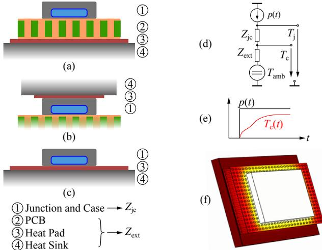
**Fig. 6:** Different switch cooling approaches and thermal modeling process. (a) and (f): Surface-mounted device cooled through the PCB or (b): directly at its case. (c): Through-hole device mounted on a heat sink. (d): Equivalent circuit for the thermal models.  $Z_{jc}$  is available from datasheets whereas  $Z_{ext}$  is extracted from the system's thermal step response (e) which is obtained using transient FEM simulations (f).
