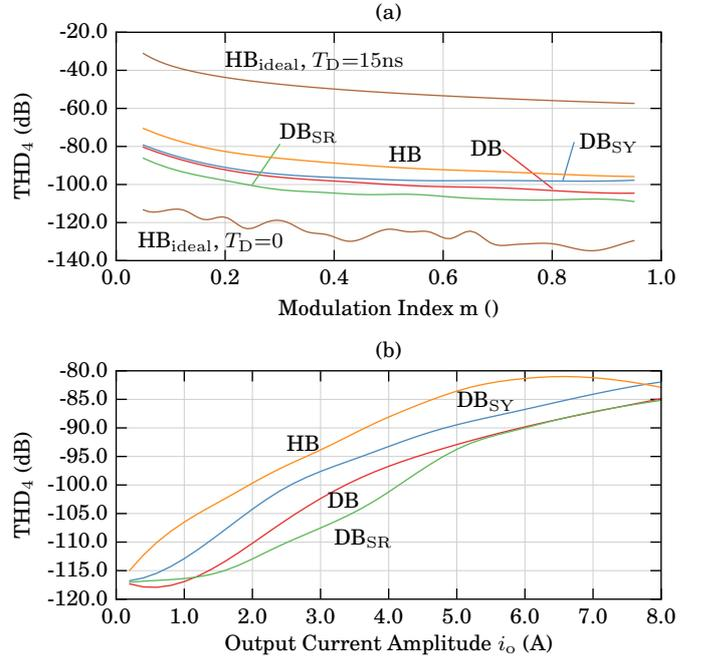
Fig. 9: Comparison of different circuit topologies with the GaN<sub>T1</sub> switch and the SiC<sub>D1</sub> diode. THD as a function of (a): the modulation index  $m$  and (b): the output current amplitude  $i_o$ .  $f_{PWM} = 100$  kHz,  $f_T = 50$  Hz,  $f_o = 2$  kHz,  $m_{nom} = 0.75$ ,  $i_{o,nom} = 3$  A,  $\varphi_o = 0^\circ$ ,  $T_{D,HB} = 15$  ns,  $T_{D,DBSR} = 15$  ns,  $I_{Off} = 5$  A,  $U_{DC} = 400$  V.
