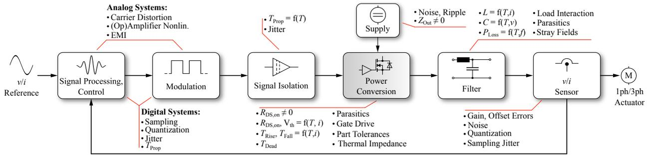
Fig. 2: Sources of output distortion in a generalized switch-mode amplifier system featuring a feedback loop. Many component properties vary with the operating point and signal time behavior (e.g., temperature or output current) of the system, rendering it nonlinear. The control and modulation blocks can be implemented using analog, digital or mixed circuitry.
