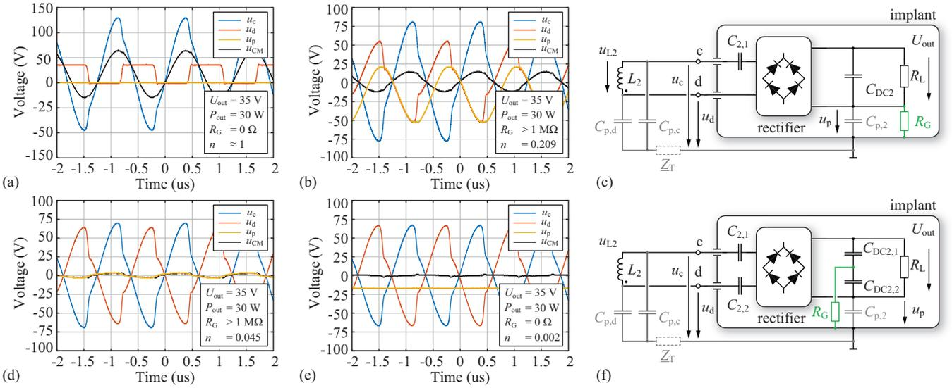
Figure 5: Results of the *in vitro* measurement of the receiver coil terminal voltages and calculated CM voltage with respect to the tissue surrounding the secondary side TET coil. (a) and (b) show the measured coil terminal voltages for the receiver topology shown in (c). (d) and (e) show the coil terminal voltages for the topology illustrated in (f).
