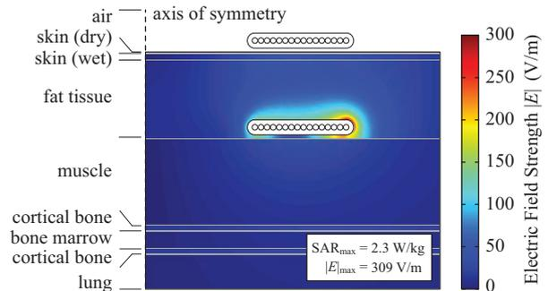
Figure 2: Simulation model geometry and simulation result of the electric field strength in the human tissue for the operating condition of the prototype TET system specified in **Tab. IV(b)** and the converter topology shown in **Fig. 1**
