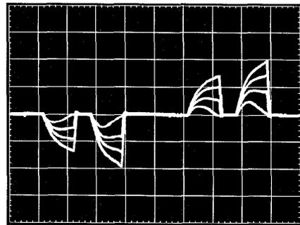
Fig. 5. Shape of a mains phase current for different values of the DC link voltage (590V/580V/570V/550V) and/or different braking power levels (9.3kW/7.2kW/5.4kW/1.6kW). Remaining operating parameters of the system according to Fig.3. Scales:20A/div, 2ms/div.
