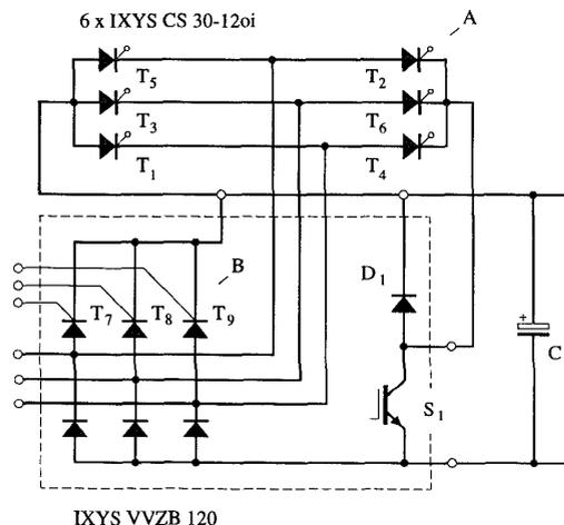
Fig. 1. Basic structure of a bidirectional input stage of a voltage DC link PWM converter drive system for application of a *Loss-Free Braking Resistor* (thyristor bridge A) for feed back of braking energy from the DC link (DC link capacitor  $C_0$ ) into the mains.
