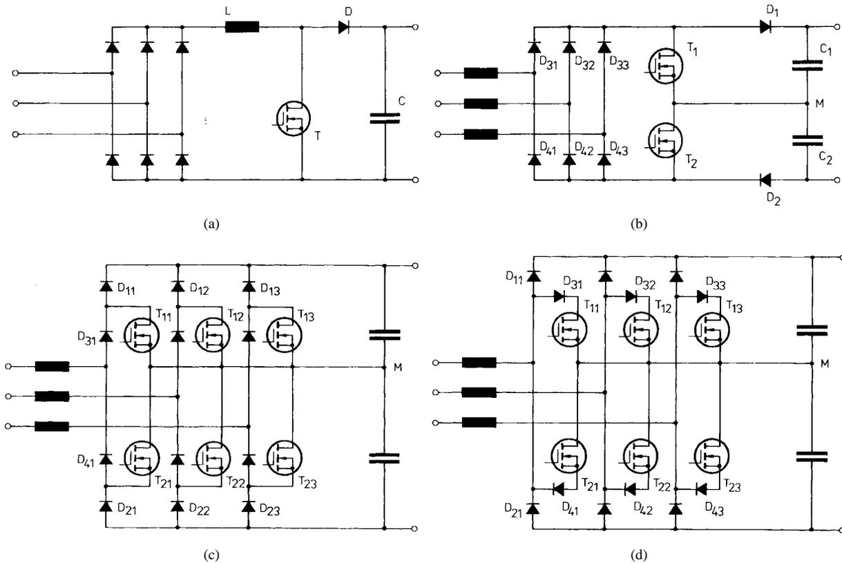
Fig. 1. Development of the basic circuit structures of three-phase three-level PWM rectifiers [(c) and (d)] based on a combination of a three-phase diode bridge and a dc/dc boost converter (a).
