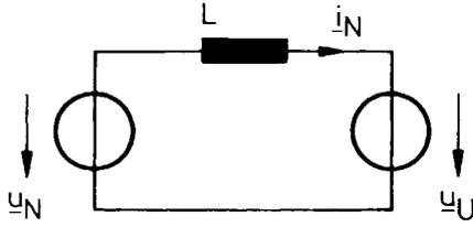
Fig. 3. Single-phase equivalent circuit related to the fundamental for the ac-side system section of a three-phase/switch/level PWM (VIENNA) rectifier.
