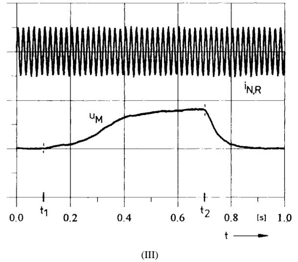
Fig. 9. (Continued.) For the control of the potential of the capacitive center point  $M$  of the output voltage. (III) Shape of  $u_M$  (100 V/div) and  $i_{N,R}$  (40 A/div) for open ( $t \in [t_1, t_2]$ ) and closed center point voltage control loop ( $\hat{I}_N^* = 18$  A, capacitance of the output capacitors  $C_1 = C_2 = 2.0$  mF). For operating parameters of the system not specified, see Fig. 7.
