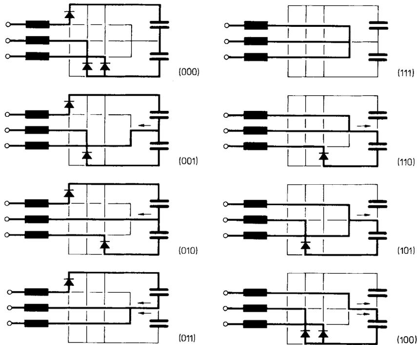
Fig. 6. Basis for the determination of the center point current  $i_M$  in dependency on the converter switching state (marked by  $(s_R, s_S, s_T)$ ) for  $\varphi_N \in (-\pi/6, +\pi/6)$  and/or  $i_{N,R} > 0, i_{N,S} < 0$ , and  $i_{N,T} < 0$  ( $i_{N,R} \geq |i_{N,S}|, |i_{N,T}|$ ).
