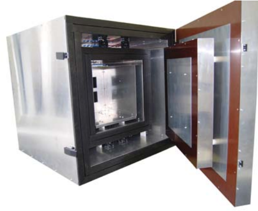
Fig. 28. Two-chamber calorimeter for high-precision measurement of the losses of power electronics converters ( \varepsilon_V < 3.5\% @10 W, < 1.0\% @100 W, < 0.5\% @200 W) developed at ETH Zurich [33], [34]; the temperature inside the inner chamber, i.e. the ambient temperature of the device under test can be set in the range T_c = T_a + 10^\circ\text{C} to 85^\circ\text{C} ( T_a is the temperature at the surface of the outer chamber).
