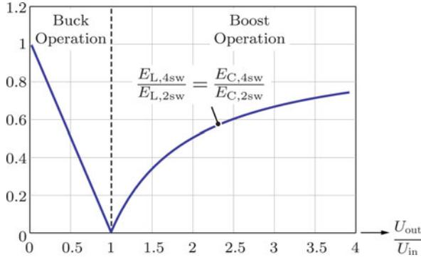
Fig. 10. Relation of the energy stored in the inductors and/or capacitors of the two-switch and the four-switch buck–boost converter under the assumption of a certain equal relative current and/or voltage ripple  $\varepsilon_{uC} = \varepsilon_{iL}$ .
