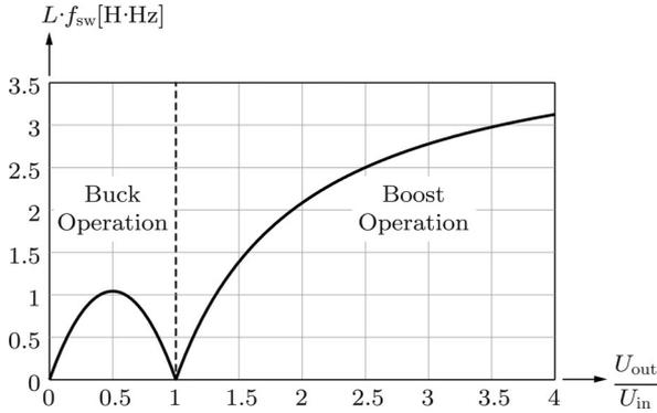
Fig. 11. Normalized inductance value in dependence of the output to input voltage ratio for an operating point of  $U_{in} = 25$  V and a maximum current ripple of  $\pm 30\%$  of  $I_{in,max}$ .
