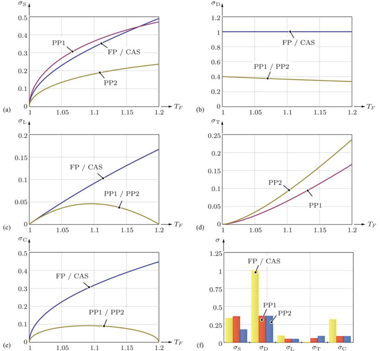
Fig. 21. CLF values of the different component types for the converters of Fig. 20: (a) transistor CLF ( $\sigma_S$ ), (b) diode CLF ( $\sigma_D$ ), (c) inductor CLF ( $\sigma_L$ ), (d) transformer CLF ( $\sigma_T$ ), and (e) capacitor CLF. In (f) the different CLF values are plotted for a transfer ratio of  $T_F = 1.1$ .
