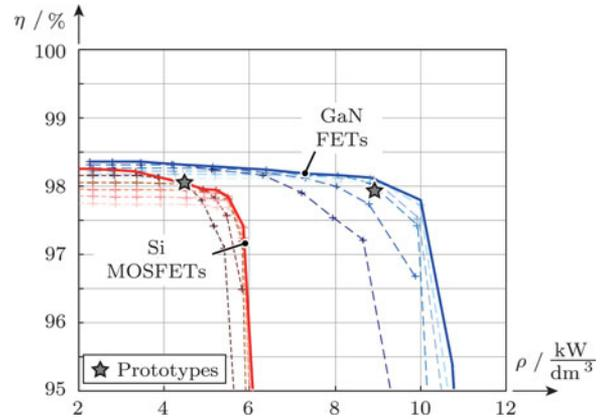
Fig. 13. Results of the  $\eta$ - $\rho$  Pareto optimization for a four-switch buck–boost converter with either Si MOSFETs or GaN FETs. The efficiency is calculated as the mean value of two operating points, i.e., at an input voltage of 30 V and an output voltage of 20 V and/or 40 V with an input power of 200 W. The solid lines represent the Pareto fronts of each semiconductor technology, whereas the dashed lines are results for specific switching frequencies (20 kHz . . . 500 kHz).
