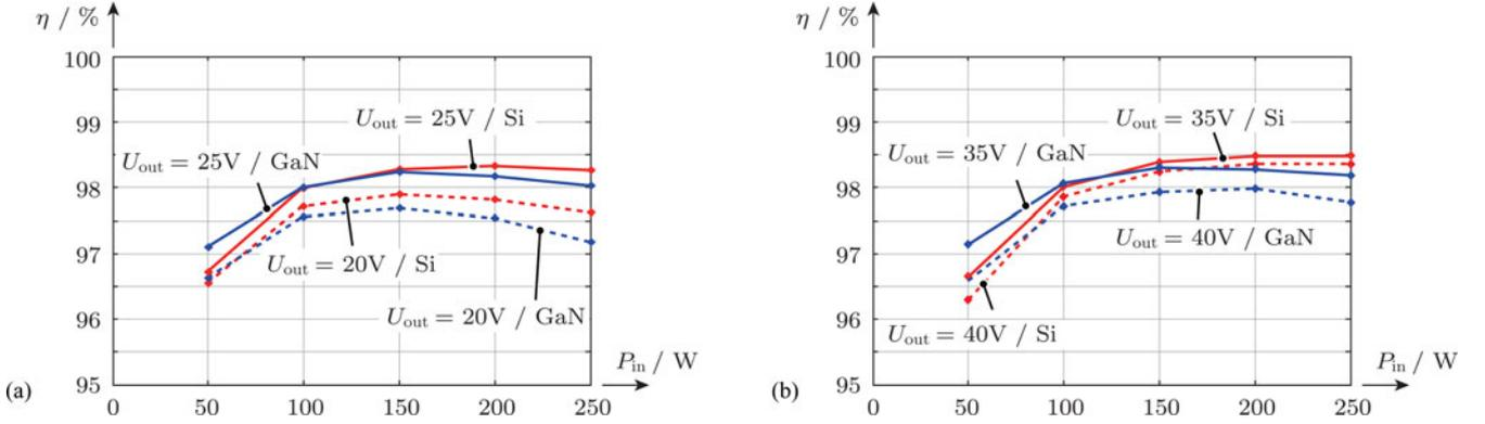
Fig. 16. Efficiency measurement results of the Si converter prototype ( $f_{sw} = 100$  kHz) and the GaN prototype ( $f_{sw} = 400$  kHz): (a) Buck operation at 30 V input voltage and output voltages of 20 and 25 V for different levels of input power  $P_{in}$  and (b) boost operation at 30 V input voltage and for output voltages of 35 and 40 V for the same levels of input power  $P_{in}$ .
