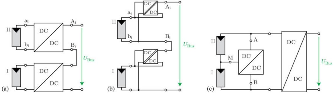
Fig. 3. Possible dc–dc converter topologies ensuring MPP operation of PV panels in series connection: (a) full-power converters, (b) series-connected partial-power converters (S-PPC), and (c) parallel-connected partial-power converter (P-PPC).
