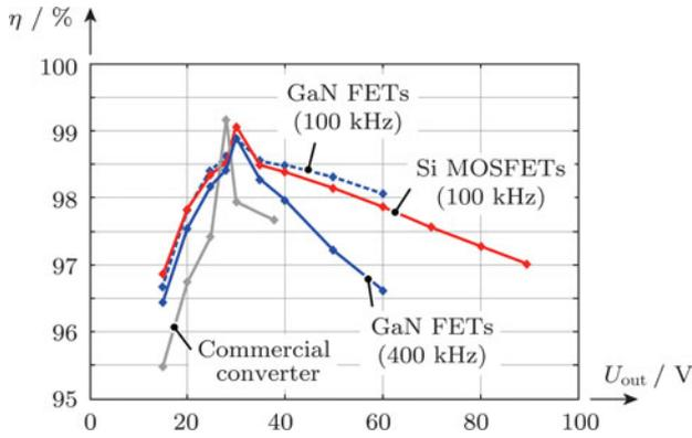
Fig. 17. Efficiency measurement results of the Si converter prototype with a switching frequency of 100 kHz, and the GaN converter with a switching frequency of 400 kHz and also with 100 kHz in comparison to a commercial PV panel-integrated buck–boost converter. The measurements were performed with an input voltage  $U_{in}$  of 30 V and an input power  $P_{in}$  of 200 W.
