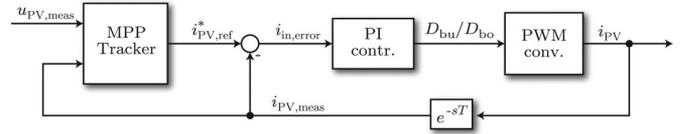
Fig. 18. Cascaded converter control with the MPP tracker as (slow) outer control loop and the PV current controller as (fast) inner control loop.
