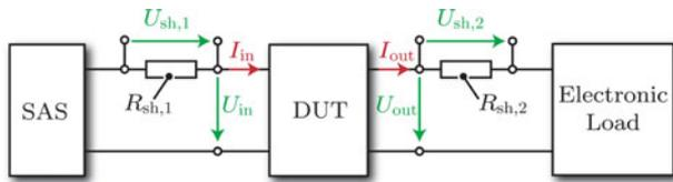
Fig. 15. High precision efficiency measurement setup comprising a solar array simulator, the converter as device under test, an electronic load, highly accurate voltmeters, and shunt resistors for current measurements.
