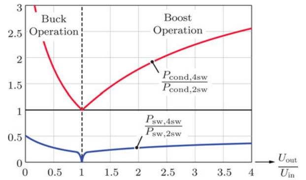
Fig. 9. Relation of semiconductor losses, i.e., conduction losses  $P_{cond}$  and switching losses  $P_{sw}$ , between the four-switch and the two-switch buck–boost converter under the assumption that the same total silicon area is used for both converter designs.
