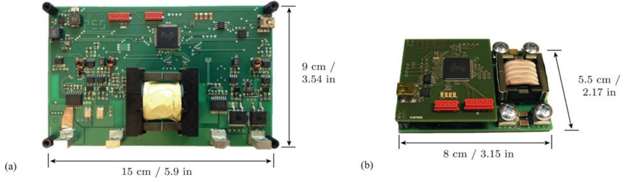
Fig. 14. PV panel-integrated buck–boost converter prototypes: (a) Prototype with Si MOSFETs (input side: IPB072N15N3/Infineon in D2Pak package, output side: BSB028N06NN3/Infineon in CanPak package) and 100 kHz switching frequency, and (b) prototype with GaN FETs (EPC2001/EPC) and 400 kHz switching frequency.
