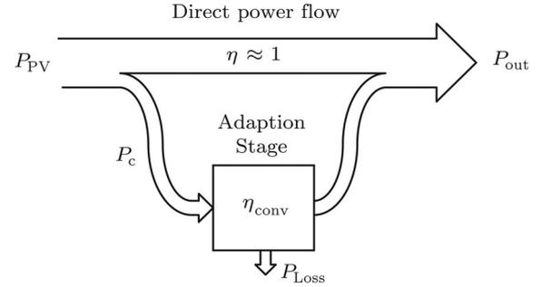
Fig. 6. Splitting of the power flow into two parallel power flow paths given for PPCs. The direct path transfers power from the PV panel to the output without any conversion stage. Only a fraction  $P_c$  of the panel output power  $P_{\text{PV}}$  is processed by a voltage (or current) adaption stage with efficiency  $\eta_{\text{conv}}$ .
