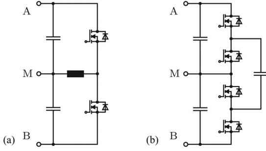
Fig. 7. Possible realizations of the parallel connected partial-power converter (P-PPC): (a) converter based on a bidirectional buck–boost converter and (b) a switched-capacitor converter.
