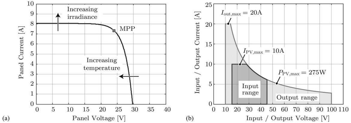
Fig. 8. (a) Influence of temperature and irradiance on electrical characteristic of PV panel and (b) derived input and output specifications of the PV panel-integrated converter.
