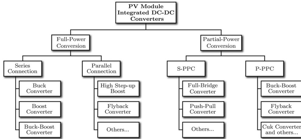
Fig. 2. Classification of PV module integrated dc–dc converter concepts into full-power and partial-power processing converters, each with subcategories of series and parallel connection.
