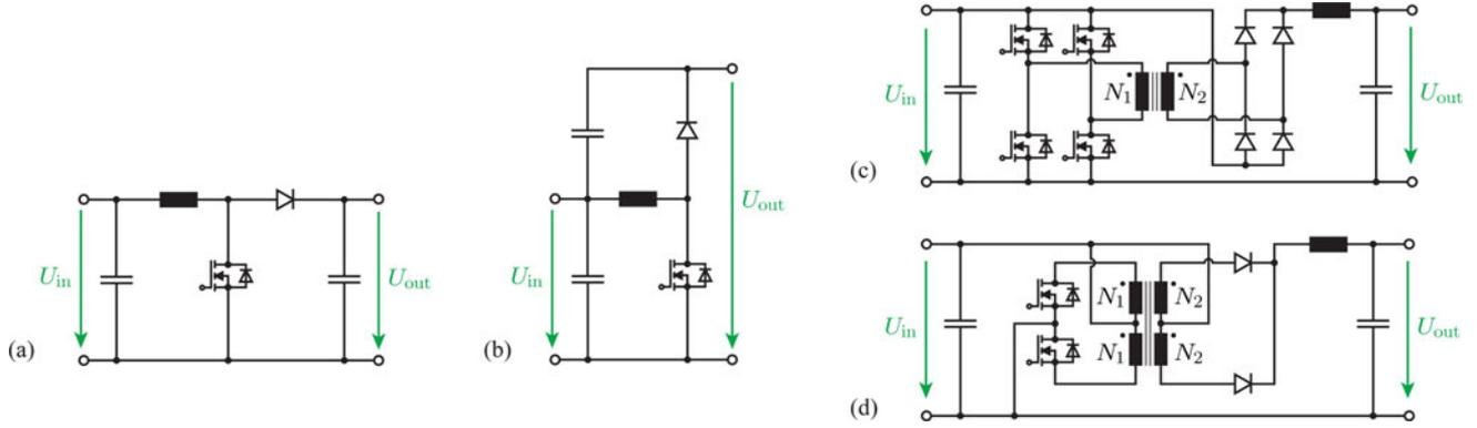
Fig. 20. Full-power and S-PPC boost converter topologies. (a) Standard full-power boost converter used as reference (label: FP), (b) cascaded S-PPC consisting of a buck-boost converter with cascaded input and output voltages (label: CAS), (c) S-PPC with a MOSFET full-bridge on primary side and full-bridge diode rectifier on the secondary side (label: PP1), and (d) S-PPC with a push-pull stage on the primary side and center-tapped rectifier on the secondary side (label: PP2).
