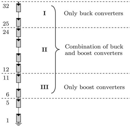
Fig. 5. Example of maximum and minimum number of PV panels per string when either only buck converters (I) or only boost converters (III) are used. The buck–boost converters combine those two regions and extend it to the previously unreachable area II. (Numbers used for this example:  $U_{\text{Bus}} = 400$  V,  $U_{\text{MPP}} = 25$  V,  $P_{\text{PV,max}} = 250$  W,  $\Delta = 1.5$ ,  $I_{\text{out,max}} = 20$  A,  $U_{\text{out,max}} = 100$  V.)
