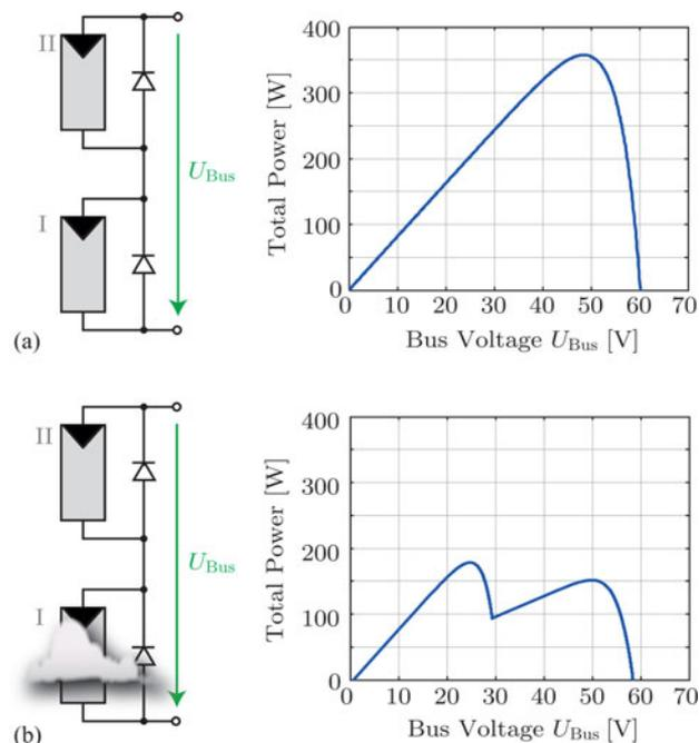
Fig. 1. Impact of shading on a simplified string formed by only two PV panels: (a) output power of the PV string with only unshaded panels receiving equal irradiance and (b) with the shaded panel (plotted versus the total bus voltage  $U_{Bus}$ ).
