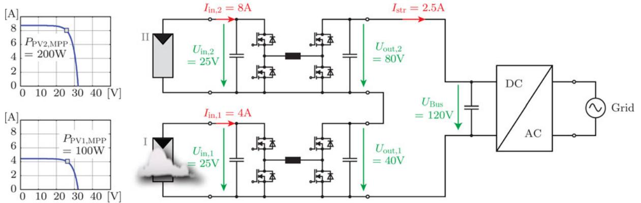
Fig. 19. Example of a PV system which employs for reasons of simplification only two PV panels with integrated buck–boost converters and generates accordingly a low bus voltage  $U_{\text{Bus}}$  of only 120 V. Each converter tracks the MPP of the attached PV panel and the central dc–ac inverter controls the bus voltage with a reference value of 120 V. The converter output voltages  $U_{\text{out},1}$  and  $U_{\text{out},2}$  reach a steady-state value according to (22).
