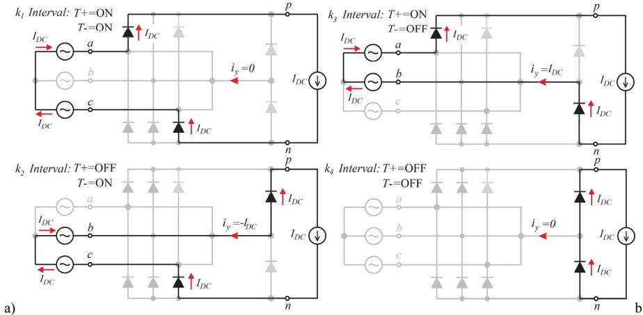
Fig. 4: a) Conduction states and b) input current space vector diagram of the SWISS Rectifier for  $\varphi_N \in [0^\circ, 30^\circ]$ .
