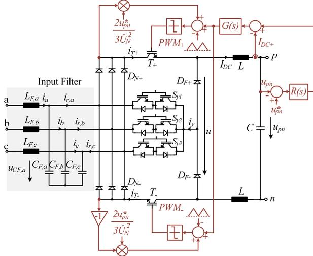
**Fig. 6:** PWM control structure for the SWISS Rectifier.
