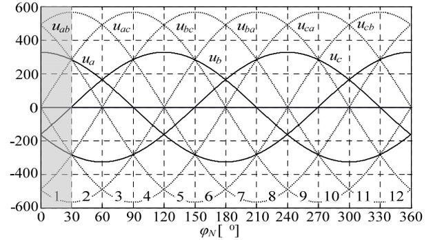
**Fig. 3:** Mains sectors 1 to 12 defined by the different relations of the instantaneous values of the mains phase voltages  $u_{a,b,c}$ .
