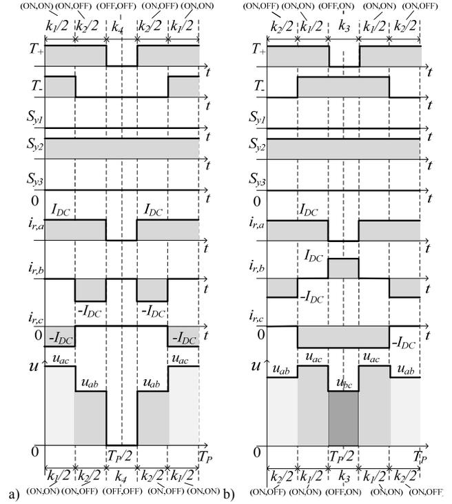
Fig. 5: Modulation scheme for a) minimal injection current ripple  $\Delta i_y$  or b) minimal dc current ripple  $\Delta i_{DC}$  for  $\varphi_N \in [0^\circ, 30^\circ]$ .
