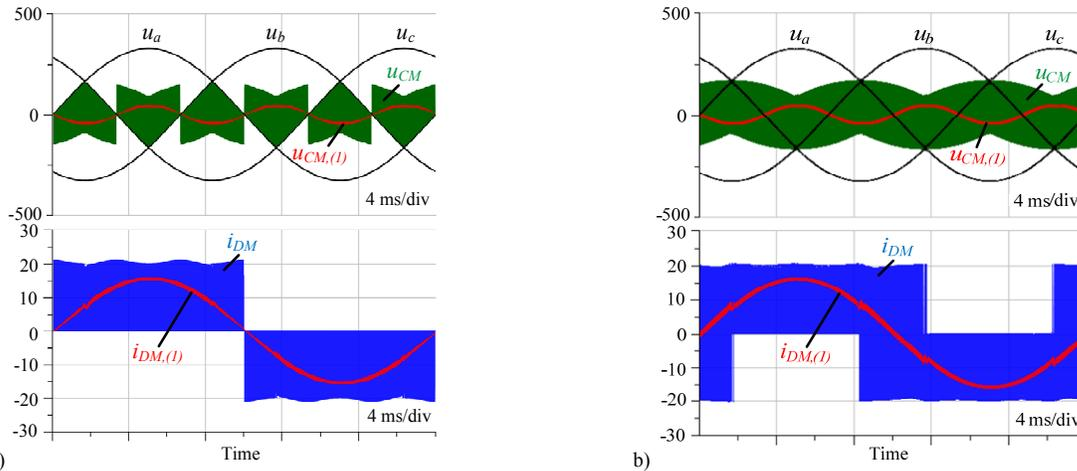
**Fig. 9:** Time behavior of the CM voltage  $u_{CM}$  and DM current  $i_{DM}$  noise sources of the SWISS Rectifier operating with modulation **a)** for minimal injection current ripple  $\Delta i_v$  [cf. Fig. 5(a)] and **b)** for minimal dc inductor current ripple  $\Delta i_{DC}$  [cf. Fig. 5(b)].
