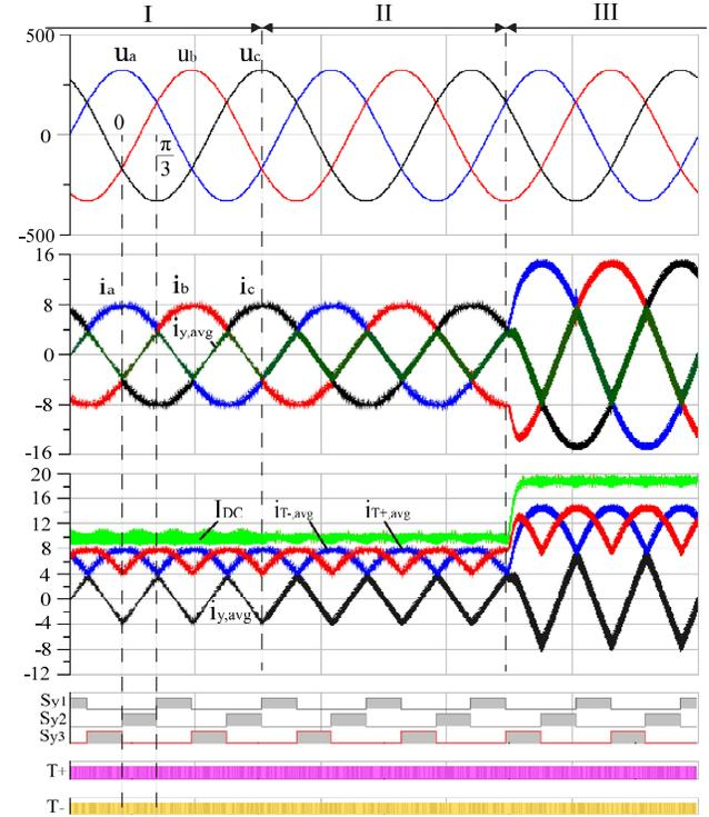
**Fig. 7:** Simulation results of the SWISS rectifier operating with (I) in-phase or (II) interleaved PWM carriers; (III) load step from 50% to 100% of the rated output power (3.75 kW to 7.5 kW).
