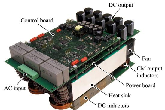
**Fig. 10:** Implemented 7.5kW SWISS Rectifier hardware prototype, using 1200 V Trench and Fieldstop IGBTs and 1200 V SiC MPS freewheeling diodes. (Mechanical dimensions: 210 mm x 132 mm x 92 mm; power density: 2.94 kW/dm<sup>3</sup> = 48 W/in<sup>3</sup>, switching frequency:  $f_p = 36$  kHz.).
