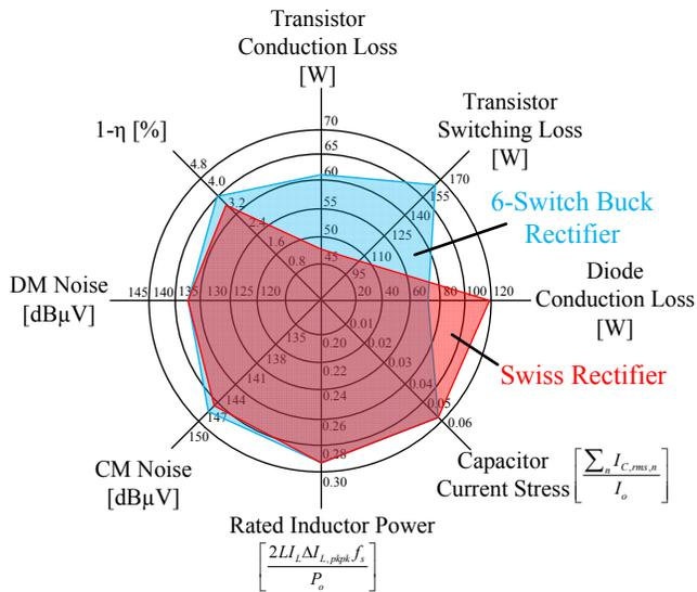
**Fig. 11:** Comparative evaluation of the Swiss Rectifier with the 6-switch buck-type rectifier. (The more advantageous system covers the smaller area in the diagram.)
