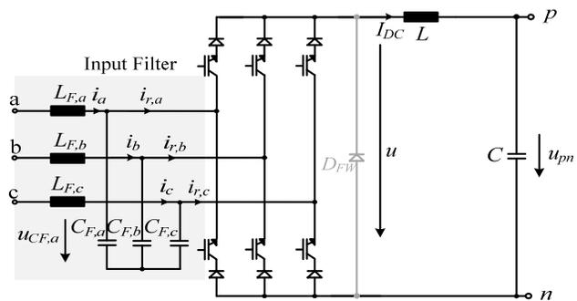
**Fig. 2:** Circuit topology of a three-phase 6-switch buck-type PFC rectifier with LC input filter and explicit freewheeling diode  $D_{FW}$ .
