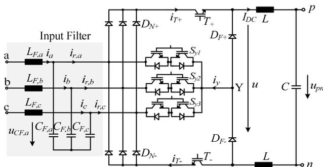
**Fig. 1:** Circuit topology of the proposed three-phase SWISS Rectifier with LC input filter.
