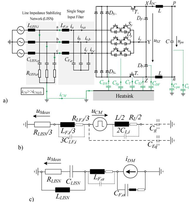
**Fig. 8:** a) Model for the propagation of the common mode currents in the SWISS Rectifier used for deriving the CM noise model. Simplified high-frequency model for b) CM and c) DM emissions, including the high-frequency equivalent circuit of the LISN and a single stage DM input filter with parasitics of inductive and capacitive elements shown.
