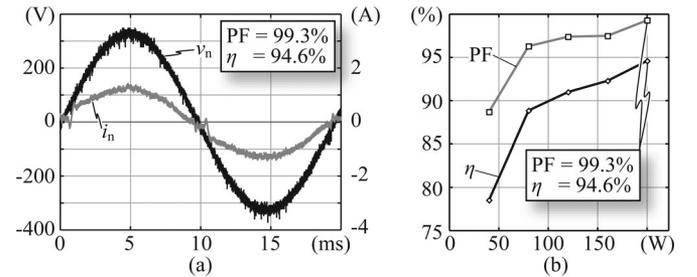
Fig. 13. (a) Input voltage  $v_n$  and input current  $i_n$  of the TCM PFC rectifier ( $V_n = 230$  V,  $V_{out} = 400$  V,  $P_{out} = 200$  W). (b) Efficiency  $\eta$  and power factor PF as a function of the output power  $P_{out}$ .
