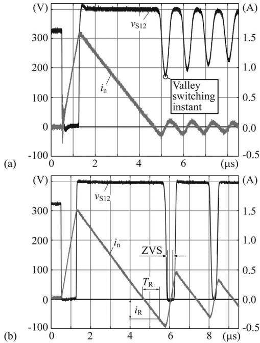
Fig. 4. Measurement results of a boost cell (a) without and (b) with an extended reverse conduction time  $T_R$  [cf., Fig. 3(b) and (c)]. In order to minimize the switching losses, (a) valley switching can be applied, whereas the extension of  $T_R$  allows for (b) ZVS over the complete mains period. (Parameters:  $v_n = 328$  V,  $V_{out} = 400$  V, and  $T_{on} = 750$  ns).
