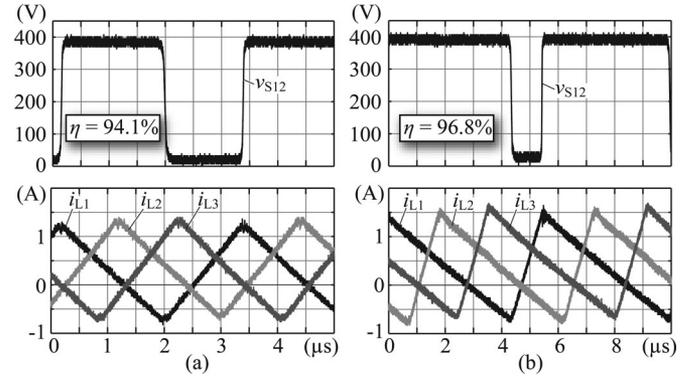
Fig. 12. Measurement results of converter system operating in dc–dc mode. The figure shows that each bridge-leg operates in ZVS mode and that the interleaving of the inductor currents is properly achieved with the presented interleaving control method. (a)  $v_n = 230$  V,  $V_{out} = 400$  V, and  $P_{out} = 200$  W. (b)  $v_n = 325$  V,  $V_{out} = 400$  V, and  $P_{out} = 400$  W.
